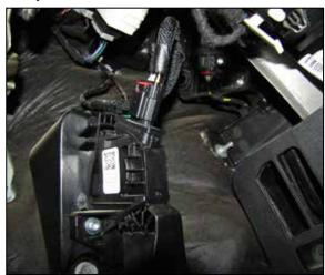
2. Locate the pedal wiring harness connection on top of the throttle pedal assembly and release the red locking tab and disconnect the electrical connection.
