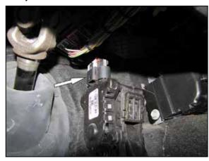
2. Release the locking tab and then disconnect the Throttle pedal electrical connection.
