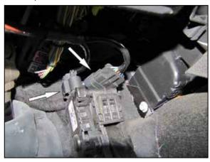
3. Connect the K&N® throttle harness to the throttle pedal and connect the factory harness to the K&N® harness.
