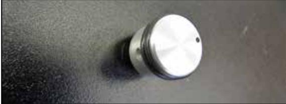
12. Find a suitable location to mount the sensitivity knob, drill a  $\frac{1}{4}$ "id hole, remove the knob and install the rheostat then reinstall the knob.
