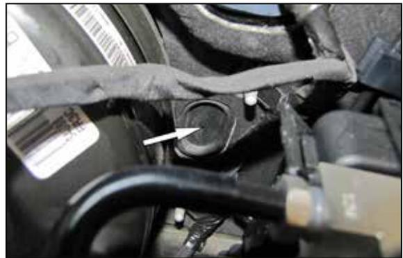
11. Poke a small hole in the existing firewall grommet and feed the boost control knob wiring harness through the grommet from the inside of the vehicle. Connect the control knob wiring harness to the pigtail connected to the module. And secure with the provided tie wraps.
