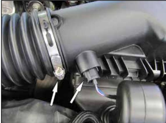
2. Disconnect the inlet air temperature sensor electrical connection. Loosen the hose clamp that secures the intake tube to the air filter housing.
