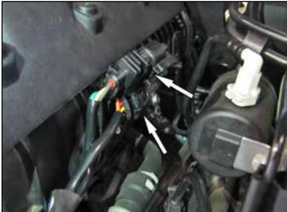
8. Connect the K&N® wiring harness to the MAP sensor and to the factory wiring harness.
