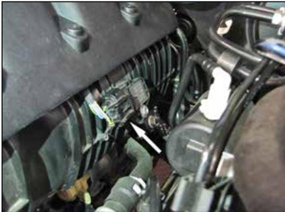
7. Locate the MAP sensor on the driver side of the engine near the engine cover. Disconnect the factory wiring harness from the MAP sensor.
