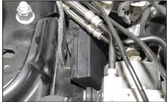
10. Mount the boost module in a suitable location such as on the back side of the shock tower as shown and secure with the provided tie wraps.
