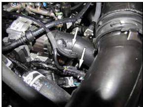
3. Disconnect the TIP sensor electrical connection and then connect the K&N® harness connectors to the TIP sensor and to the factory harness.
