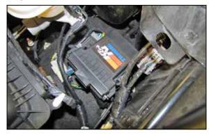
6. Mount the boost module in a suitable location such as under the brake master cylinder as shown using the provided tie wraps.
