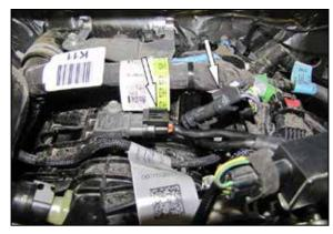
5. Connect the K&N® harness to the MAP sensor and to the factory harness. Route the K&N® harness towards the driver's side inner fender. Secure the harness with the provided tie wraps. Reinstall the decorative engine cover.
