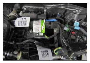
4. Disconnect the MAP sensor electrical connection at the rear of the intake manifold.
