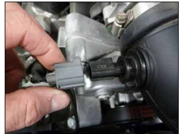
3. Disconnect the IAT sensor electrical connection.
