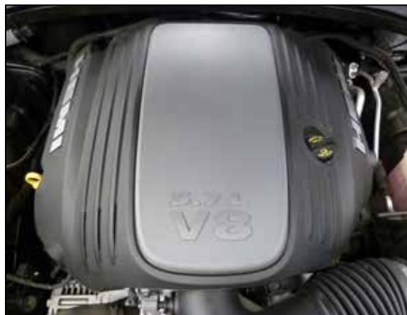
2. Lift the engine cover up and remove it from the vehicle.
