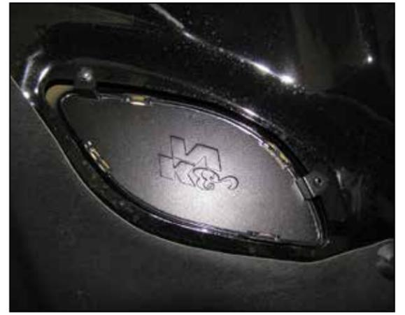
26. Install the block off and secure with the factory hardware. Jeep models will use the EPDM block off.
