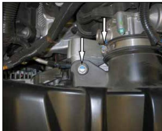
3. Remove the intake plenum mounting bolt shown and loosen the intake tube hose clamp.
