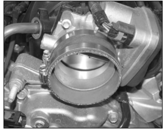
17. Install the provided silicone hose (08630) onto the throttle body and secure with the provided hose clamp.
