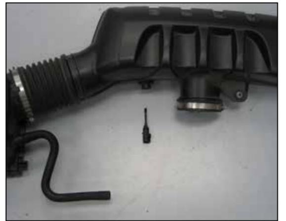
18. Release the locking tab and then remove the inlet air temperature sensor from the factory intake tube by twisting counter clockwise. **NOTE: The inlet air temperature sensor is very fragile; take care to avoid damage while handling the sensor.**
