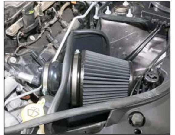
16. Install the K&N filter onto the adapter and secure with the provided hose clamp.
