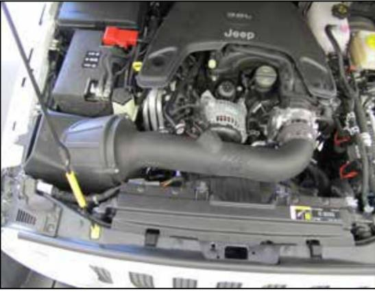
17. Install the K&N intake assembly into the hose at throttle body first, then engage the K&N airbox mounts into the factory airbox mounting location. Secure K&N intake assembly with provided clamp.
