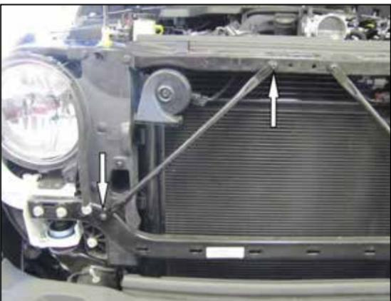
7. Remove the two bolts that secure the core support brace to the core support and remove brace. **NOTE: the brace will be reinstalled in a later step.**
