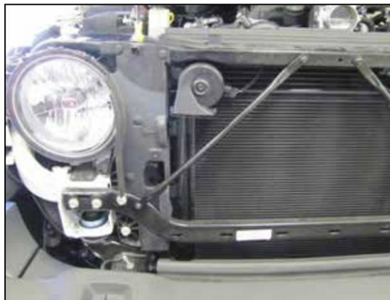
9. Reinstall core support brace onto the core support.
