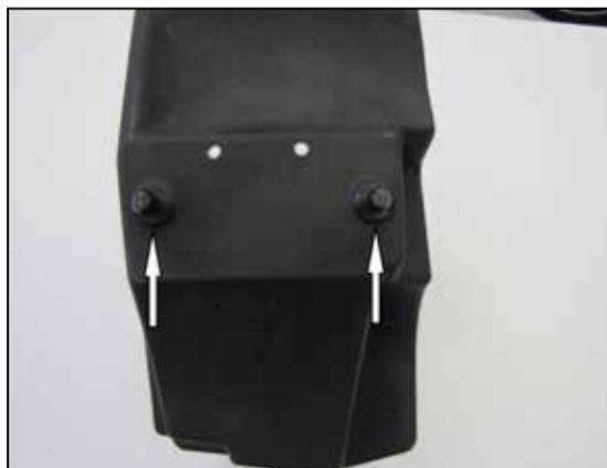
11. Install two airbox mounts onto the K&N airbox with provided hardware.
