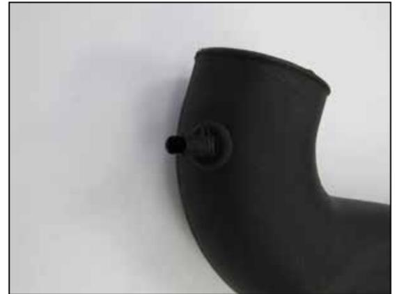
13. Remove the inlet air temp sensor from the factory inlet tube. Then remove the "O" ring from the sensor. Install the provided grommet onto the K&N intake tube. Then install the inlet air temp sensor into the grommet.
