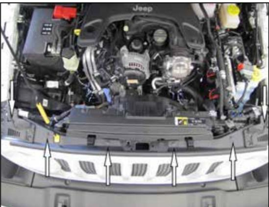
6. Remove the 6 clips at the top of the grill that secure grill to core support. Before removing grill note the location of the 8 clips that hold the lower part of the grill to the core support. Start at either side of the grill. Grasp the bottom part of the grill pulling firmly straight back dislodging the clips one at a time. Work your way across the grill until all clips have been dislodge and remove the grill.
