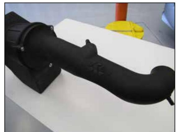
15. Install the K&N intake tube assembly onto the K&N airbox with provided hardware. **NOTE: the orientation of the K&N intake tube.**
