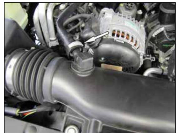
3. Disconnect the crank case vent line.
