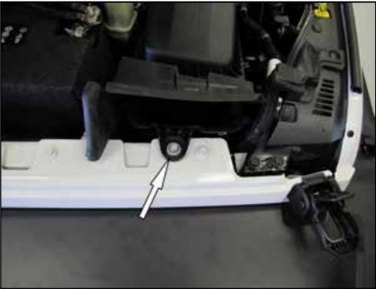
5. Remove the bolt that secures the factory air box to the filter and remove assembly.
