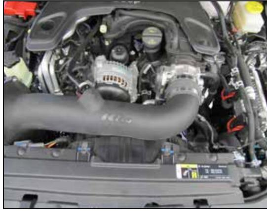
18. Reconnect the crank case vent line onto the quick connect fitting and reconnect the inlet temp sensor electrical connector onto the temp sensor.
