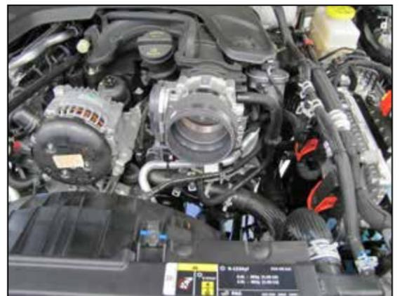
16. Install provided hose onto the throttle body (08171) secure with provided clamp.
