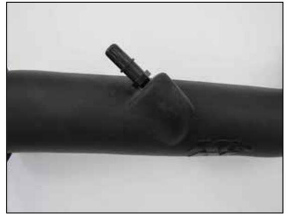
12. Install 1/4 NPT quick connect fitting onto the tube.
