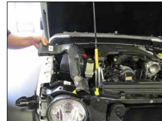
8. Remove the two bolts that secure the inlet scoop to the core support and remove inlet scoop.
