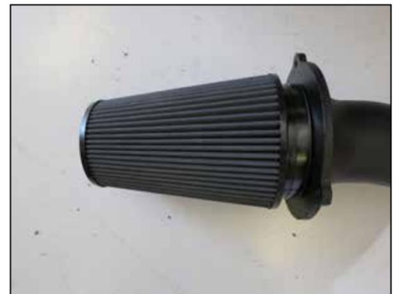
14. Install the K&N air filter onto the K&N intake tube.
