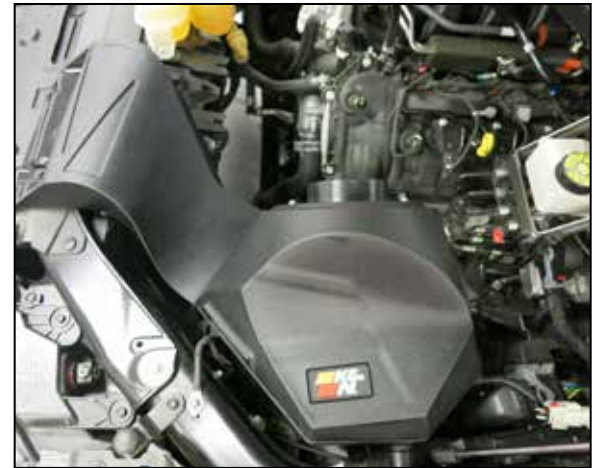
18. Install the upper housing assembly onto the lower housing so the mounting posts insert into the grommets.
