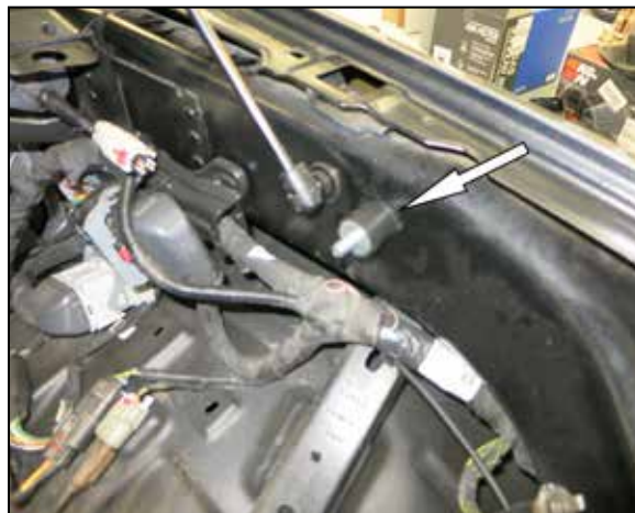
11. Install the provided rubber mounted stud into the inner fender at the air filter housing mounting location.
