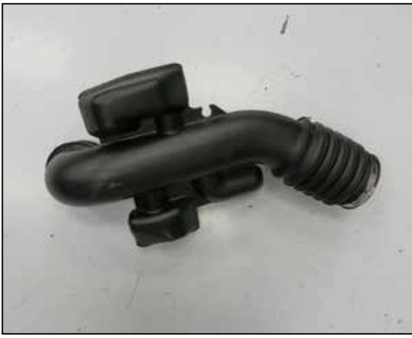
4. Remove the intake tube from the vehicle.
