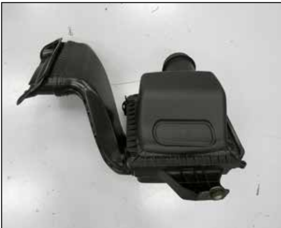
7. Remove the air filter housing/fresh air intake duct assembly from the vehicle.
