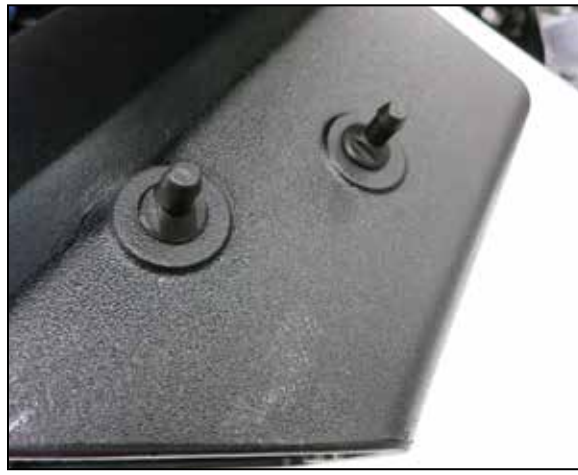
9. Install the provided mounting studs onto the K&N lower air filter housing using the provided hardware.
