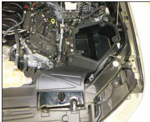
12. Install the K&N lower air filter housing assembly into the vehicle.
