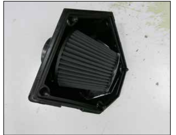
17. Install the K&N air filter onto the adapter and secure with the provided hose clamp.
