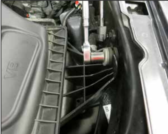
6. Remove the bolt that secures the factory air filter housing to the inner fender.
