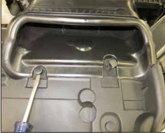
5. Pry up the push-pin locks that secure the fresh air intake duct and remove the pins.
