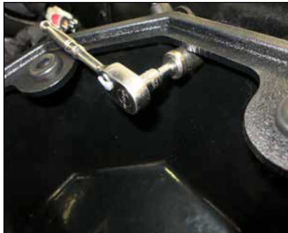
13. Secure the housing to the rubber mounted stud from step #11 with the provided hardware.
