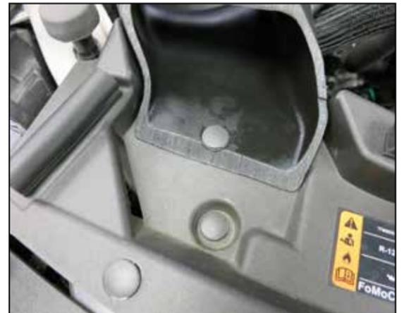
32. Install the factory push-pin to secure the fresh air intake duct.
