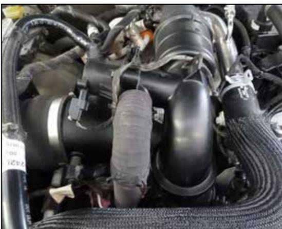
24. Install the BOV hose onto the BOV fitting. Do not secure with the spring clamp currently.
