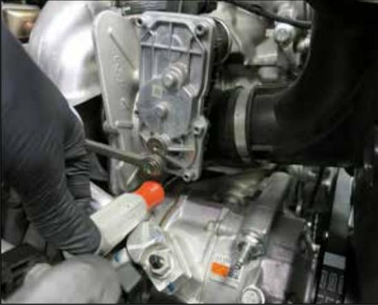
9. Loosen the hose clamp that secures the factory intake tube to the turbo.
