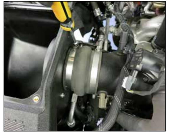
30. Connect the intake tube to the coupler and secure with the hose clamp.
