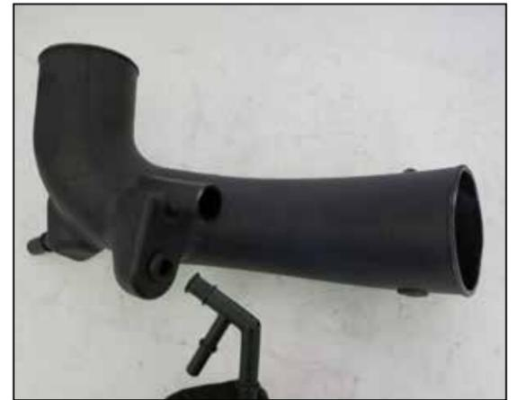
18. Install the provided Ejector fitting into the grommet in the K&N intake tube as shown. **NOTE: use care while installing the Ejector fitting, grip the main section of the body just above where the grommet meets the stop bead. Pushing down on the top 45 degree section may result in the fitting to fracture at the junction to the straight section.**
