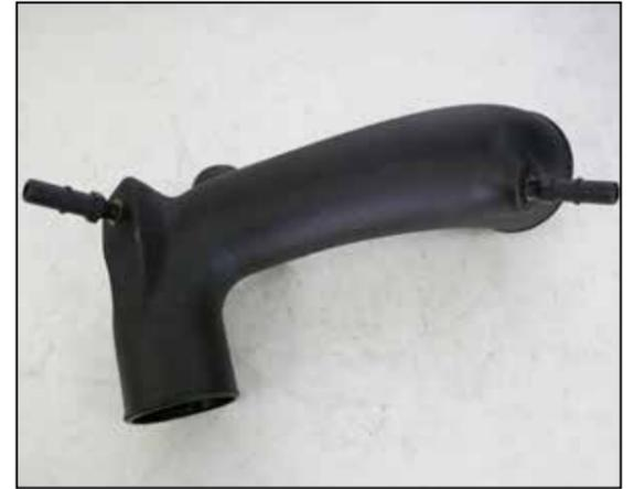
17. Install the two provided quick connect fittings into the K&N intake tube as shown.
