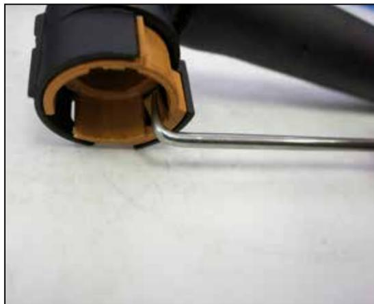
13. Disconnect the CCV hose from the valve cover. There are three clips inside the connector that lock the fitting onto the valve cover, using a 90-degree pick the clips can be released one at a time while applying slight pressure upwards on the fitting. The upward pressure will help prevent the clips from relocking while releasing the others. Replacement connectors are provided to be used with the K&N intake kit.
