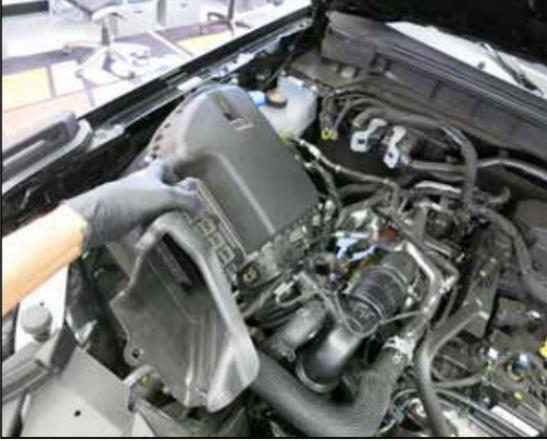
8. Remove the factory air filter assembly from the vehicle.
