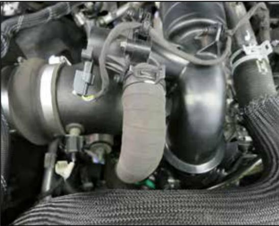
36. Secure the BOV hose to the BOV valve with the factory hose clamp.
