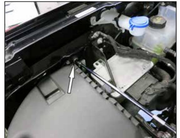
5. Remove the bolt that secures factory air filter housing to the inner fender.
