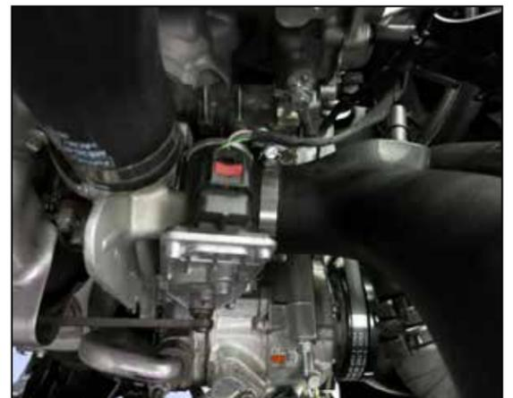
33. Tighten the hose clamp that secures the intake tube to the turbo inlet.
