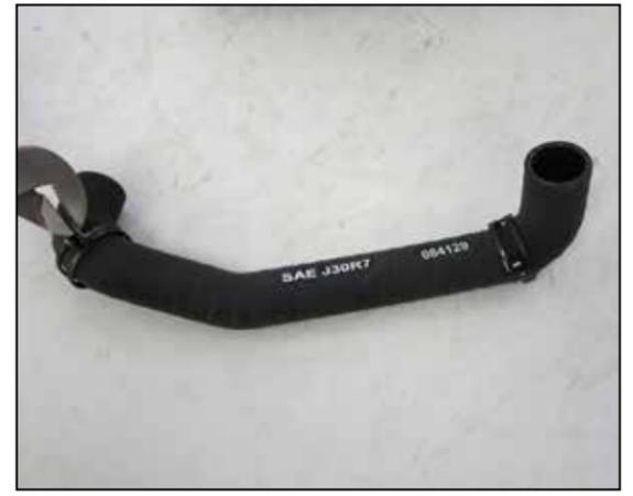
15. Remove the factory BOV spring clamps from the factory BOV hose and install them onto the provided BOV hose.
