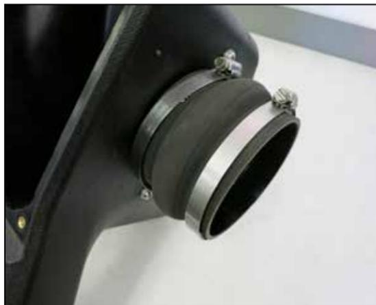
28. Install the provided filter adapter into the K&N air filter housing and secure with the provided hardware. Install the provided hump coupler onto the filter adapter and secure with the hose clamp.
