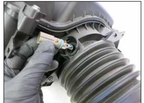
19. Rotate the IAT sensor counterclockwise and up to remove it from the factory air filter housing.
