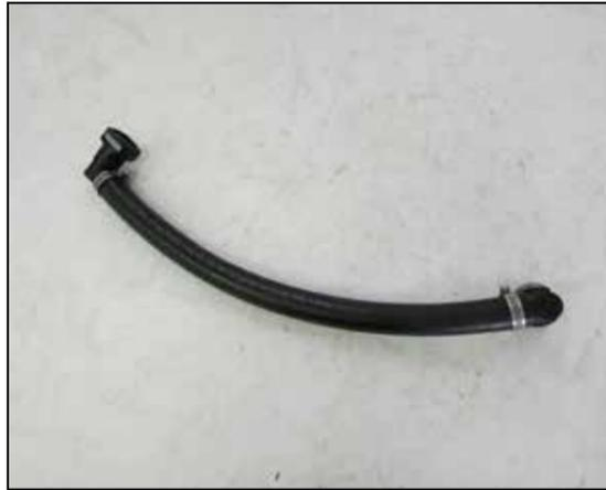
26. Assemble the CCV hose with the provided quick connect fittings as shown.
