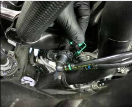
11. Remove the green locking clip that secures the larger EVAP hose to the Ejector fitting and then disconnect the hose.
