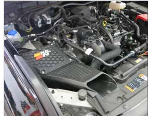
41. Reconnect the negative battery cable. Double check to make sure everything is tight and properly positioned before starting the vehicle. **NOTE: With the K&N intake system install you will notice more noise from the intake system, turbo charger and blow valve system. You will hear air escaping and the BOV pop on deceleration. This is normal.**
