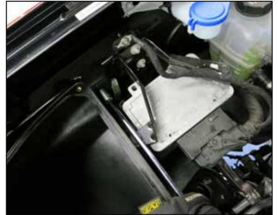
31. Secure the air filter housing to the inner fender with the provided bolt.
