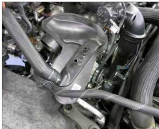
14. Remove the factory intake tube assembly.
