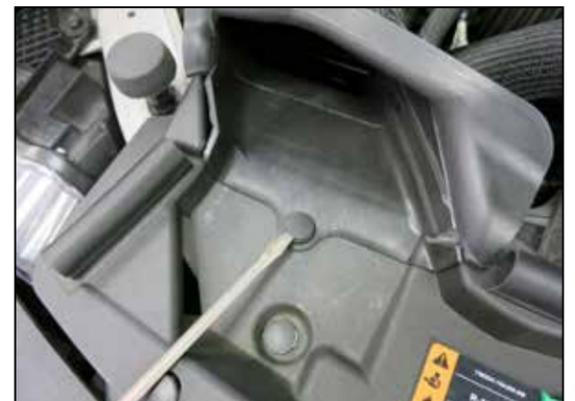
6. Remove the push-pin that secures the fresh air intake duct.
