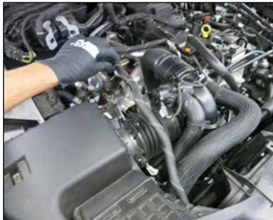
3. Separate the coolant line from its mounting point on the factory air filter housing.
