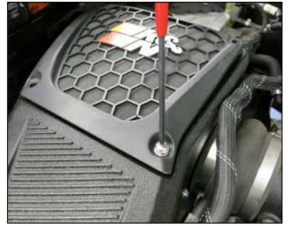
39. Install the prefilter onto the air filter housing and secure with the provided hardware.
