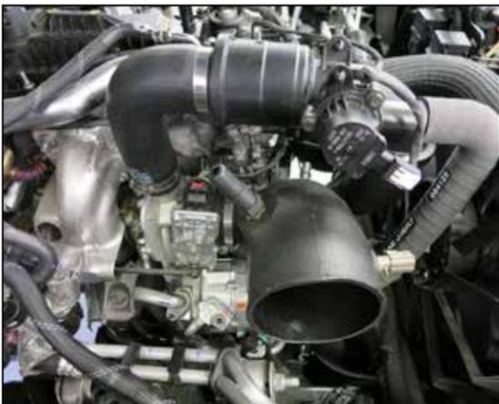
23. Install the K&N intake tube assembly onto the turbo inlet but do not secure the hose clamp.
