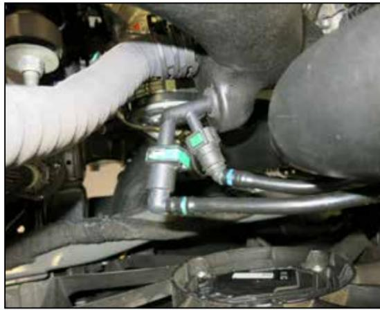
25. Reconnect the Ejector hoses onto the ejector installed into the K&N intake tube.
