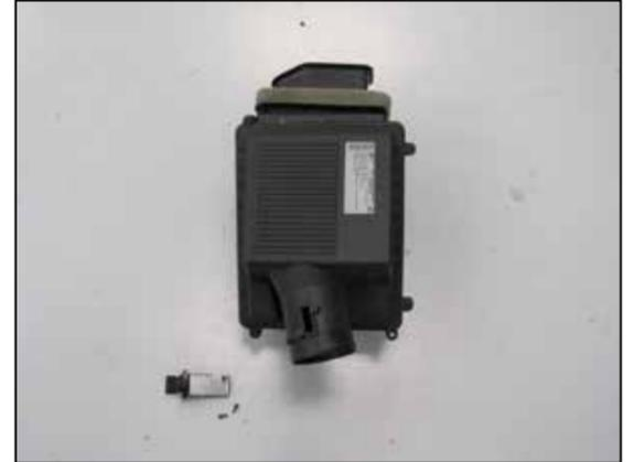
16. Remove the mass air sensor from the factory air box.
