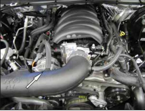
21. Connect the provided crank case vent hoses to the ports on the valve covers and then connect the open ends to the fittings installed into the K&N intake tube.
