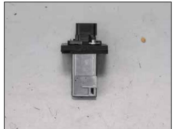
17. Install the mass air sensor into the K&N adapter and secure with the provided hardware.
