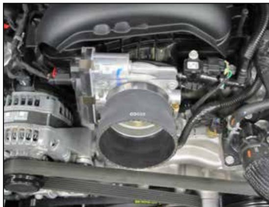
13. Install the coupling hose (08497) to the throttle body and secure with the provided hose clamp.
