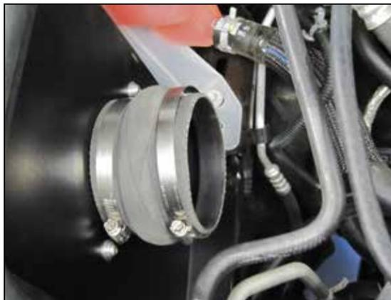
14. Install the coupling hose (08418) to the filter adapter and secure with the provided hose clamp.
