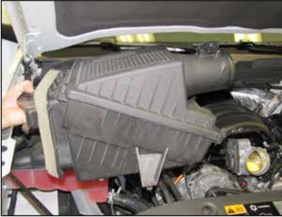
6. Pull up the air box to release it from the mounting grommets and then remove the factory air box from the vehicle. **NOTE: It will be necessary to unhook the mass air sensor wiring harness from the air box as it is removed.**
