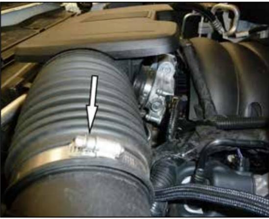
4. Loosen the hose clamps that secures the intake plenum to the air filter housing and to the throttle body. Disconnect the plenum connections at the air filter housing and then rotate the plenum counter clockwise to disengage the keyed mount and separate it from the throttle body. **NOTE: The wiring harness anchored to the intake plenum will need to be detached before removing the plenum from the vehicle.**
