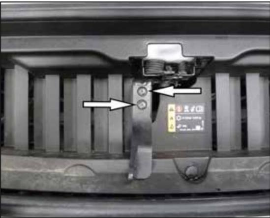
5. Remove the two bolts that secure the hood release arm to the hood latch and then remove the arm.
