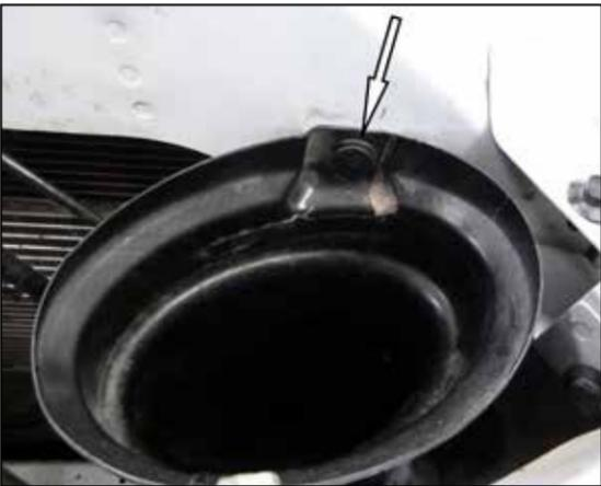
7. Remove the plastic retaining clip that secures the fresh air intake duct to the core support, then pull the duct forward to disengage it from the factory air filter housing.
