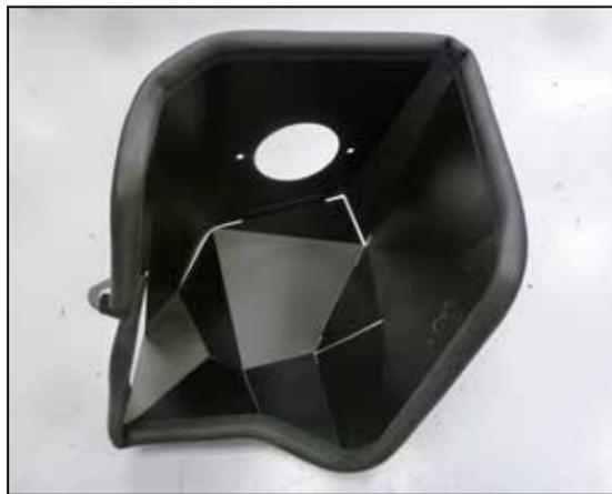
10. Install the provided edge trim onto the heat shield as shown. **NOTE: Some trimming of the edge trim will be necessary.**
