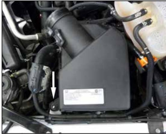
9. Remove the nut that secures the air filter housing. Unhook the wiring harness from the filter housing and then remove the air filter housing from the vehicle. **NOTE: Go slow and use caution to remove the housing. It is indexed into two holes in the rear with rubber grommets that can fall off easily and be lost. It is a tight fit but will come out without being forced. This nut will be reused in a later step.**
