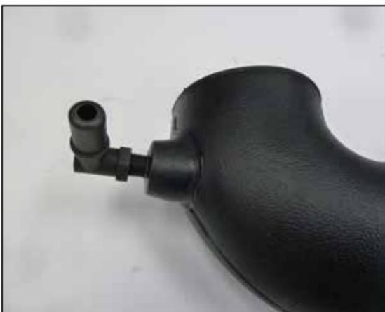
19. Install the provided 90° quick connect fitting into the K&N intake tube as shown.
