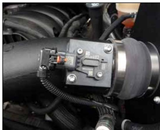
25. Connect the mass air sensor electrical connection.
