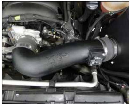
22. Install the intake tube into the coupler at the filter adapter and then into the coupler at the throttle body, adjust the tube for best fit and then secure with the provided hose clamps.
