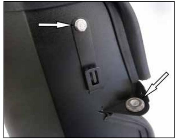
12. Install the provided wiring connector mounting bracket onto the heat shield using the provided hardware. Remove the factory mounting grommet and sleeve from the factory air filter housing and install it into the K&N heat shield as shown.
