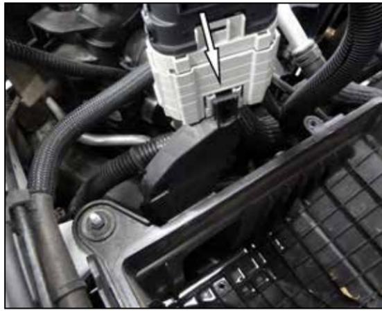
8. Using a small 90° pick or similar tool, release the locking tab that secures the wiring harness bulk connector to the air filter housing and then unhook the connector from the housing. **NOTE: The filter housing lid was removed for the purpose of this picture.**
