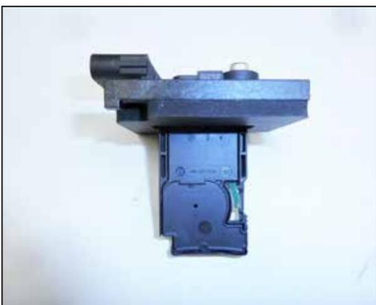
20. Install the provided gasket onto the K&N mass air adapter. Remove the mass air sensor from the factory housing and install it into the mass air adapter and secure with the provided hardware.
