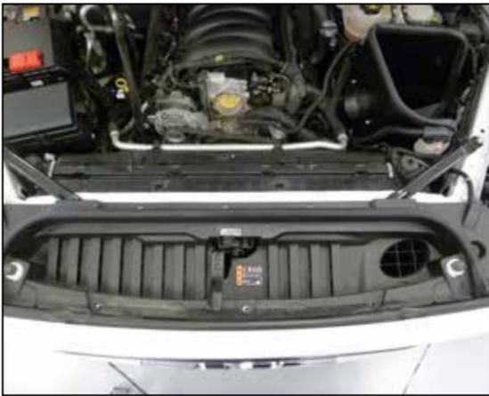
16. Reinstall the radiator valence and secure with the ten factory clips. Reinstall the hood release arm and secure with the factory hardware.
