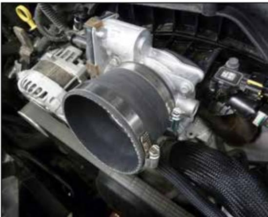
18. Install the provided reducer coupler onto the throttle body and secure with the provided hose clamp. **NOTE: On 5.3L equipped vehicles use coupler #08497, on 6.2L vehicles use coupler #084107.**
