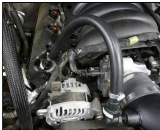
24. Connect the crank case vent hose assembly to the valve cover port and then to the fitting installed into the intake tube.
