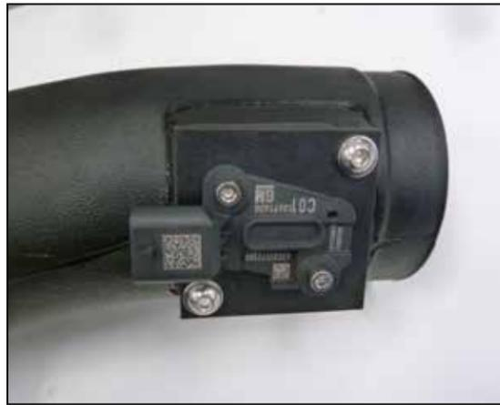
21. Install the mass air sensor into the K&N intake tube and secure with the provided hardware.
