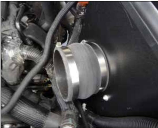
17. Install the provided hump coupler onto the filter adapter and secure with the provided hose clamp.
