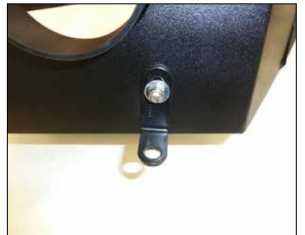
16. Install the provided mounting bracket (070712) onto the heat shield and secure with the provided hardware.
