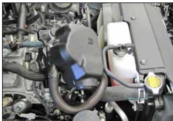
12. Lift up the air injection pump, disconnect the electrical connection and then set the air injection pump over to side.
