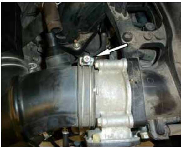
7. Loosen the hose clamp which secures the intake tube to the throttle body.
