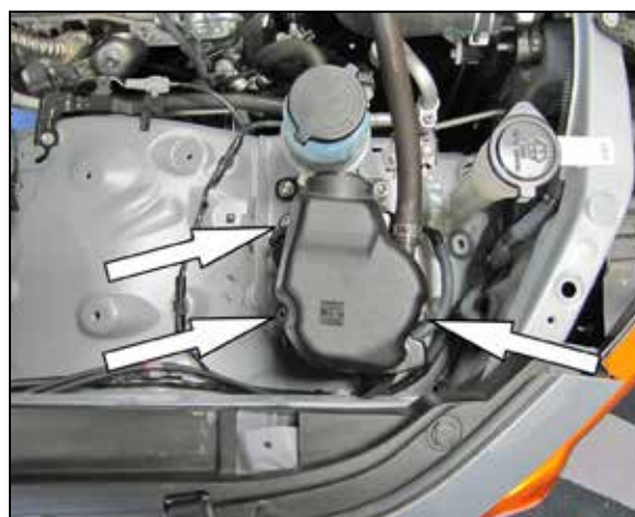
11. On models with the Air injection pump located in front of the air box next to the Power steering reservoir, remove the three bolts securing the pump to the inner fender.
