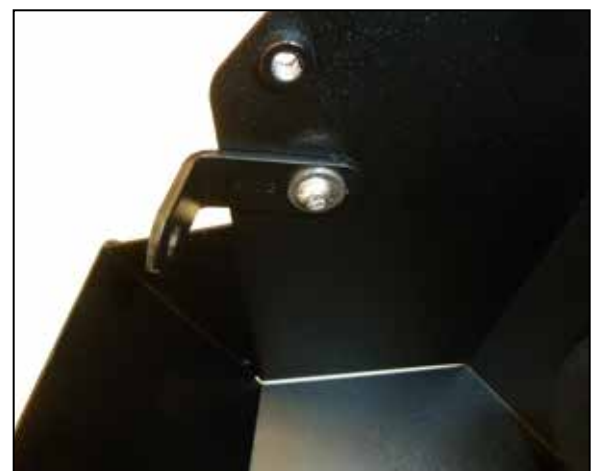
17. Install the provided mounting bracket (08022) onto the heat shield and secure with the provided hardware.
