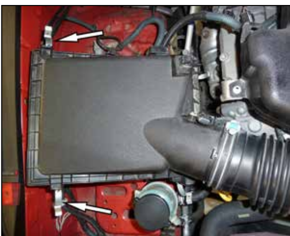
8. Release the four clips which secure the upper air box to the lower air box and then remove the intake tube and upper air box from the vehicle.
