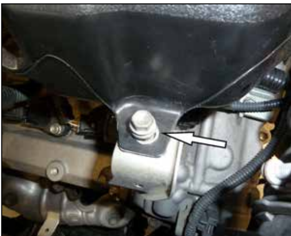
6. Remove the bolt which secures the tube mounting bracket to the engine valve cover.
