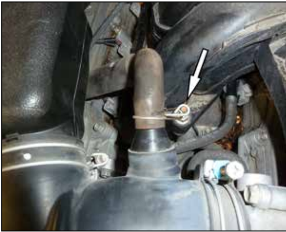
5. Disconnect the crank case vent hose from the stock intake tube.
