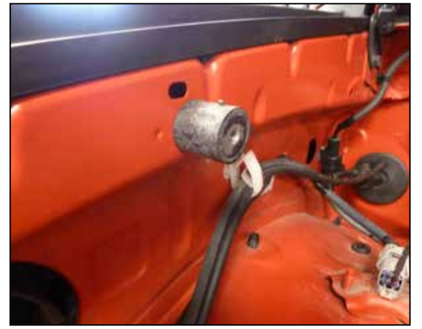
14. Install the 6mm rubber mounted stud into the inner fender location shown.
