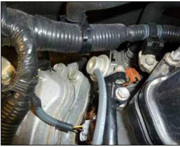
4. Unhook the fuel pressure vent line from the fuel pressure regulator.
