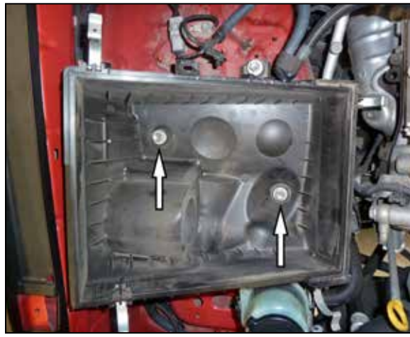
9. Loosen and remove the three bolts securing the lower air box and then remove the lower air box from the vehicle.
