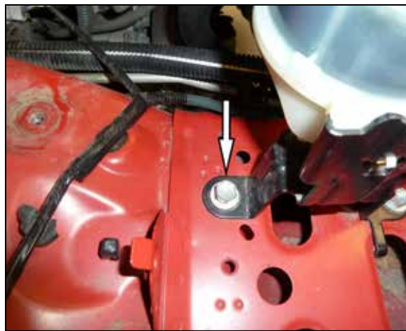
10. Remove the rear P/S reservoir mounting bolt shown.
