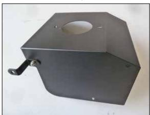
9. Install the provided heat shield bracket (07958) onto the K&N heat shield as shown.
