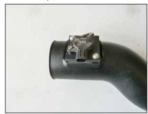
18. Install the mass air sensor assembly into the K&N intake tube and secure with the provided hardware. **NOTE:** be sure to install the sensor in the correct direction, the arrow will point towards the direction of air flow.
