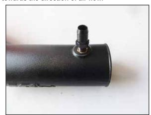
19. Install the provided vent fitting into the K&N intake tube as shown.
