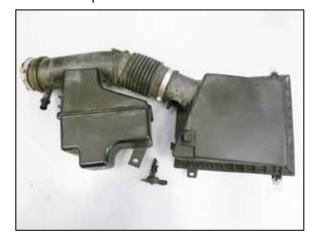
16. Remove the mass air sensor from the factory air filter housing.
