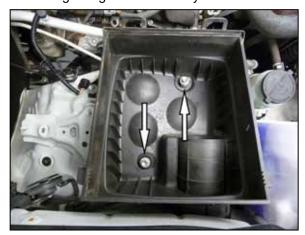
7. Remove the three bolts securing the lower air filter housing to the inner fender and then remove the lower air filter housing from the vehicle.
