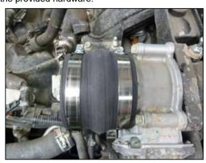
13. Install the provided coupler (01871) onto the throttle body and secure with the provided hose
