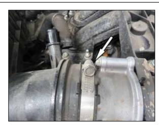
4. Loosen the hose clamp securing the factory intake tube to the throttle body.
