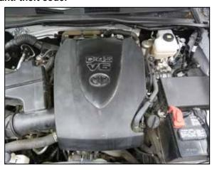
2. Lift up the engine cover to dislodge it from the mounting studs and then remove it from the vehicle.
