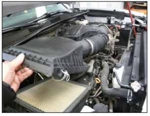
6. Release the two clips securing the upper air filter housing and then remove the intake tube and air filter hosing along with the factory air filter.
