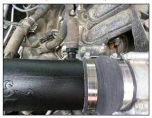
21. Connect the crank case vent fitting onto the vent fitting installed into the K&N intake tube.
