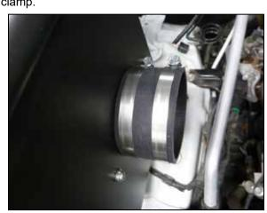
14. Install the provided coupler (08698) onto the filter adapter and secure with the provided hose clamp.
