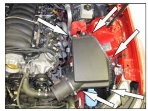
6. Release the five retaining clips and then remove the upper air box assembly.
