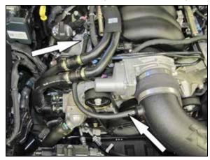
12. Connect the provided crank case vent hose to the fitting installed into the K&N® intake tube and then connect the open end to the port on the valve
