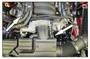
4. Disconnect the crank case vent hose from the intake plenum and valve cover and then remove the hose from the vehicle.
