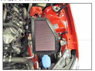
7. Replace the air filter with the provided K&N® performance air filter and reinstall the upper air box assembly. Secure the upper air box assembly with the five factory retaining clips.
