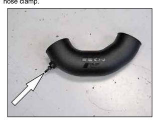
10. Install the provided vent fitting into the K&N® intake tube as shown.
