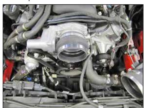
9. Install the provided hump coupler hose (08418) onto the throttle body and secure with the provided
