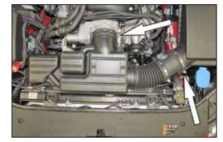
5. Loosen the hose clamps securing the intake plenum to the throttle body and to the mass air sensor then remove the plenum from the vehicle. NOTE: K&N Engineering, Inc., recommends that customers do not discard factory air intake.
