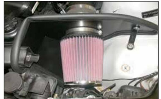
23. Install the air filter onto the mass air sensor and secure with the provided hose clamp.
