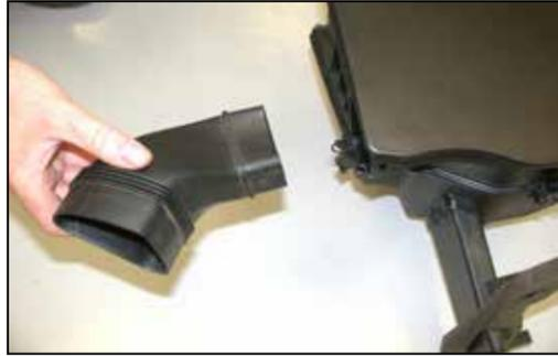
15. Remove the fresh air duct from the air box as shown.
