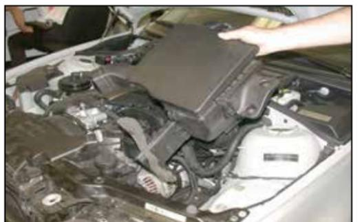
6. Lift the air box from the rear and remove it from the vehicle.
