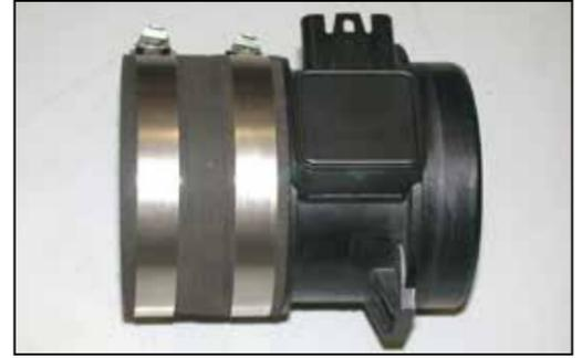
20. Install the silicone hose (08630) onto the mass air sensor and secure with the provided hose clamp.
