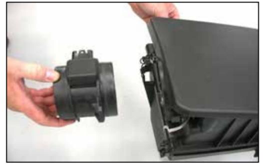
19. Unhook the two mass air sensor retaining clips and remove the mass air sensor from the air box.
