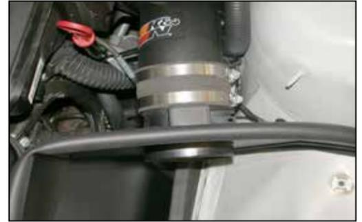
21. Install the mass air sensor assembly into the heat shield and onto the K&N® intake tube, secure with the provided hose clamp.
