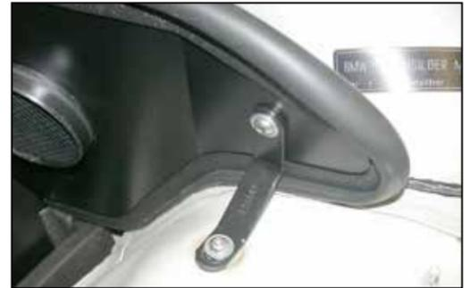
22. Secure the provided bracket (010087) onto the heat shield and inner fender with the provided hardware as shown.
