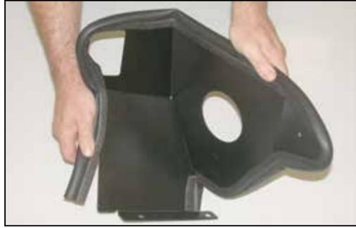
14. Install the provided edge trim onto the heat shield as shown.
