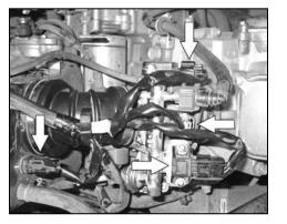
4. Unhook the four fuel injection electrical connections shown and place the wiring harness to the side guest from the intele base.
