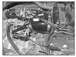
9. Reconnect the fuel injection electrical connections.
