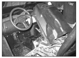
3. Lift up the engine cover and remove it from the vehicle as shown. It will be necessary to push the shifter boot through the engine cover as it is removed.
