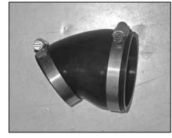
7. Install the provided hose clamps onto the K&N<sup>®</sup> silicone hose (084096) as shown.
