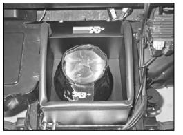
26. Install the K&N<sup>®</sup> air filter assembly onto the intake tube and secure with provided hose clamp.
