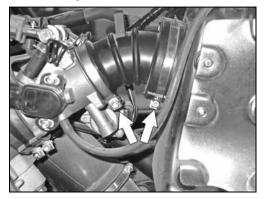
5. Loosen the two hose clamps which secure the stock intake hose to the throttle body and air chamber.
