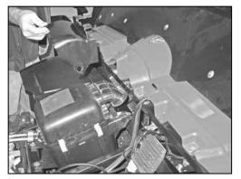
13. Remove the deflector shield as shown.
