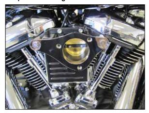
8. Using the provided throttle body mounting bolts, install the base plate onto the engine. Do not completely tighten the bolts; they are just being used to hold the base plate in the correct position at this time. Secure the servo cover to the back of the base plate with the hardware provided. Now install the remaining breather O-rings into the base plate and secure the base plate with the provided breather bolts. Then remove the three throttle body bolts.
