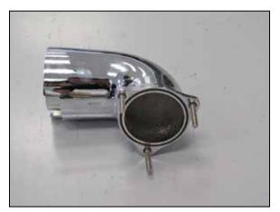
9. Install the provided O-ring and tube mounting bolts into the intake tube as shown.
