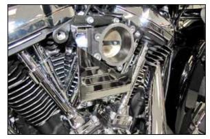
6. Install the K&N<sup>®</sup> servo cover and secure with the provided hardware to the original servo cover mounting bolt locations.
