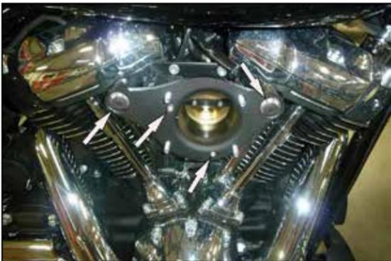
10. Using the two provided crankcase breather bolts; install the back plate onto the vehicle. Do not tighten bolts at this time. Then secure with the two other bolts provided. Tighten all bolts at this time.
