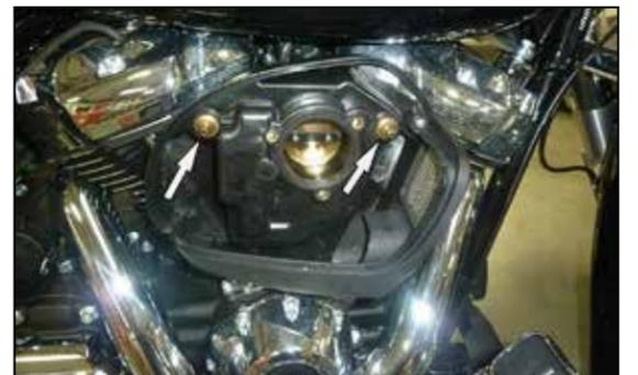
5. Remove the two breather/air filter base mounting bolts as shown.
