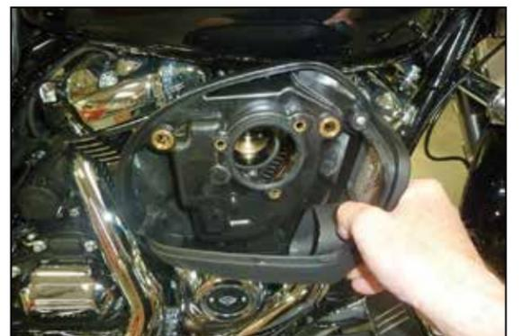
6. Remove the air filter base from the vehicle as shown.
