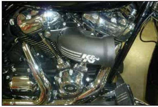
11. Install the K&N® intake tube with the gasket and provided hardware.
