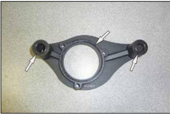
7. Install three of the o rings provided onto the back side of the K&N® back plate as shown. A small amount of grease maybe used to hold the o rings in place.
