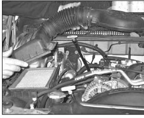
5. Remove the intake plenum and airbox.
