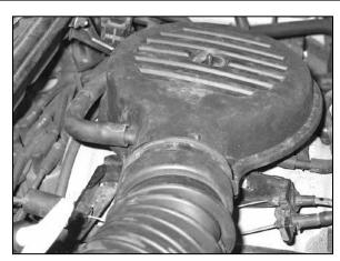
4. Remove the crankcase vent hose from intake plenum.
