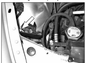
12b. Durango models only, mount the long "C" bracket (070682) to the existing hole with hardware provided.
