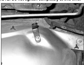
13. Secure the long "L" bracket (070662) to the airbox mounting stud.
