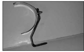
18. Assemble the saddle and angled "L" bracket using the hardware provided.
