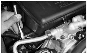
7. Loosen and remove the 2 bolts that retain the intake tube to the intake manifold.
