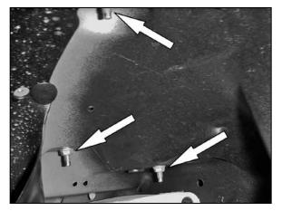
10. Loosen and remove the 3 nuts that retain the airbox base to the inner fender apron.
