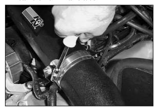
23. Secure the intake tube to the saddle bracket using the hose clamp provided.
