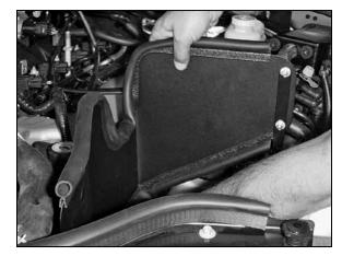
15. Install the heat shield assembly.
