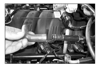
9a. On 03 models, detach the 90 degree hose from crankcase vent as shown.
