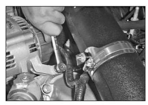
25. Tighten the alternator retaining bolt.
