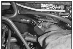
26. Attach the vent hose provided to the "T" fitting.
