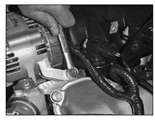
19. Loosen and remove the alternator retaining bolt.
