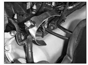
20. Attach the saddle bracket assembly to the alternator using the bolt removed in the previous step.
