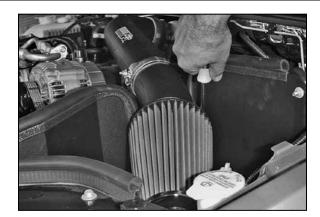
28. Install the K&N® Air Filter onto the intake tube and tighten hose clamp provided.
