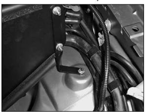
16. Attach the "L" twist bracket to the existing airbox mounting point on the inner fender apron using the hardware provided.
