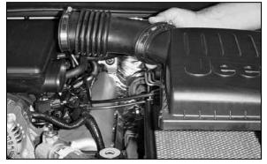
5. Detach the intake hose from the intake tube and remove the entire upper airbox assembly.
