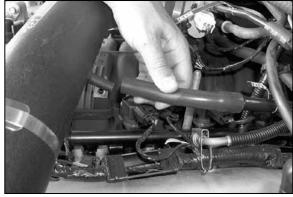
27a. On 03 models, use the 6 inch hose cut in step 27. Connect one end to crankcase vent and the other end to the intake tube as shown.
