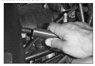
27. Attach the vent hose to the vent fitting on the K&N® intake tube.
