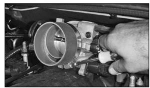
21. Attach the silicone hose to the throttle body using a hose clamp provided.
