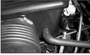
2. Detach the crankcase vent hose from the stock intake tube.
