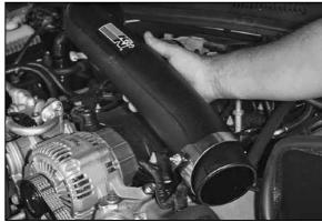
22. Install the K&N® intake tube.
