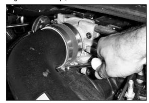
24. Tighten the hose clamp on the silicone hose at the intake tube.
