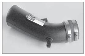
17. Install the silicone hose and hose clamps onto the new intake tube.
