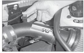
23. Reconnect the air temperature sensor electrical connection.
