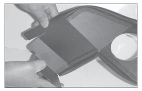
10. Install the edge seal to the heat shield as shown.
