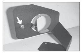
11. Mount the saddle bracket assembly to the heat shield (as shown).
