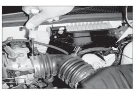
4. Loosen the hose clamps on the air intake tube at the throttle body and air box.
