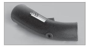
15. Install the grommet into the new intake tube.
