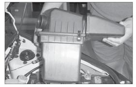
7. Lift firmly up on the air box to remove from the car.
