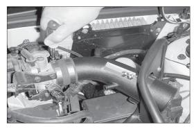
18. Install the air intake tube onto the throttle body.
