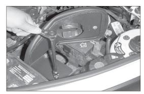
13. Install the heat shield with hardware provided (as shown).
