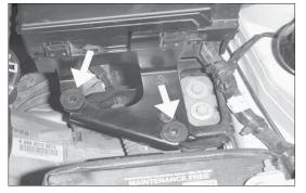
12. Install the rubber nut insert into air box grommet holes.
