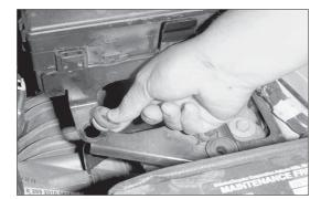
8. Remove the stock air box grommets from the stock air box mounting tray.
