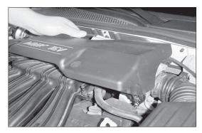
3. Pull firmly up on the engine cover to remove.
