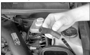
18. Remove the stock rubber hose from the EVAP canister vent line as shown.
