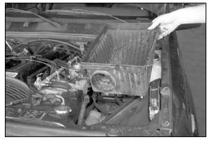
6. Remove the lower air cleaner assembly and fresh air intake tube.
