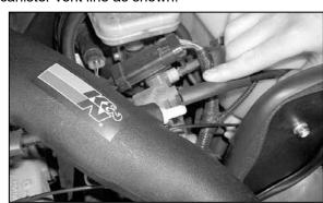
19. Install the new silicone hose onto the EVAP canister vent line and install the other end onto the K&N® intake tube as shown.
