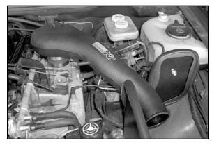
15. Install the K&N® intake tube onto the throttle body then tighten the hose clamp.
