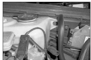
13. Using the bolt that was removed in step 11, secure the small "L" bracket onto the inner wheel well
