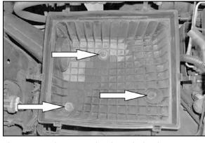
5. Loosen and remove the three bolts that secure the lower air cleaner assembly.
