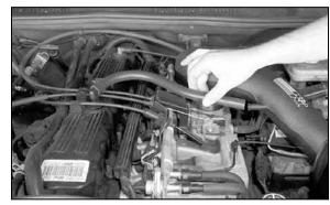
16. Install the provided silicone hose onto the crankcase vent on the valve cover, then install the other end onto the K&N® intake tube.
