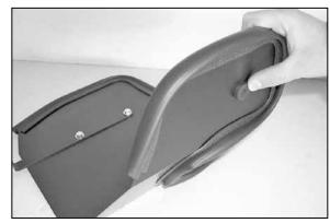
9. Install the rubber step grommet onto the heat shield as shown.
