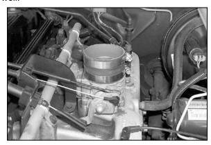
14. Install the silicone hose and the hose clamps onto the throttle body as shown.
