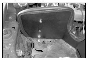
12. Install heat shield assembly into vehicle as shown. Using the hardware provided, secure large "L" bracket onto vehicle inner wheel well.
