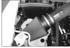
19. Install the K&N® Filtercharger onto the new K&N® intake tube as shown.
