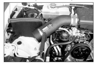
18. Install the new K&N® intake tube onto the resonator, position the intake tube for proper clearance then tighten hose clamps at the resonator and saddle bracket.
