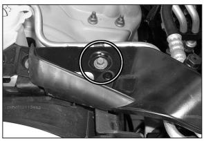
7. Remove the 6mm bolt from core support.
