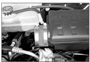
17. Install the provided silicone hose onto the resonator with the provided hose clamps as shown.
