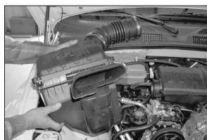
3. Firmly lift up to disengage air box from retaining grommets and remove air box from vehicle.
