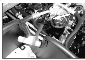
15. Install the "Z" bracket onto the A/C compressor and secure with the bolt that was removed in step 13.
