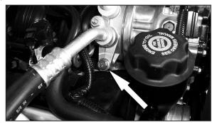
13. Remove the A/C compressor-mounting bolt.
