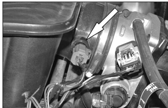
4. Depress the locking tab on the air temperature sensor electrical connection and then pull to disconnect the sensor electrical connection.
