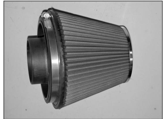
25. Install the filter adapter into the Air filter as shown and secure with the provided hose clamp.
