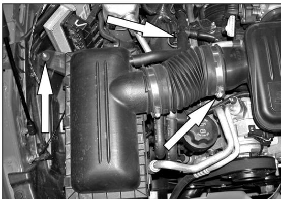
2. Loosen the hose clamp at the throttle body and the air box mounting nut, and then disconnect the crank case vent hose from the "tee" fitting.
