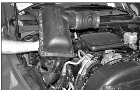
3. Disconnect the stock intake tube from the intake plenum and lift to remove the air box assembly from the vehicle as shown.
