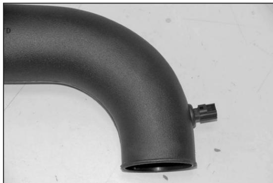
21. Install the sensor into the grommet installed in step #18.
