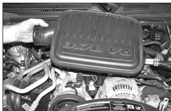
5. Lift to dislodge the intake plenum from its mounting grommets and remove the intake plenum from the vehicle as shown.
