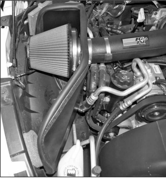
27. Install the Air filter assembly onto the K&N® intake tube and secure with the provided hose clamp as shown.
