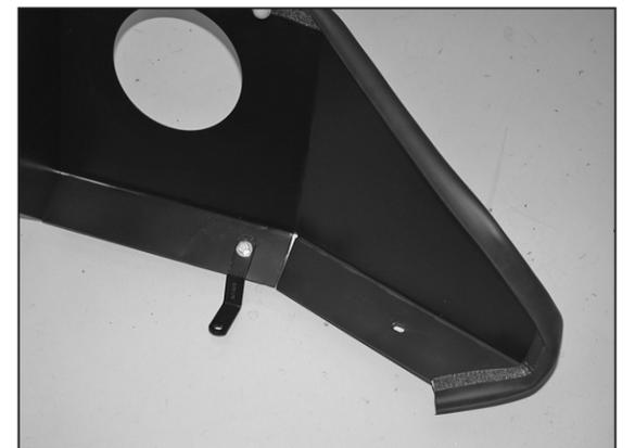
9. Install the "Z" bracket (010120) onto the heat shield with the provided hardware as shown.
