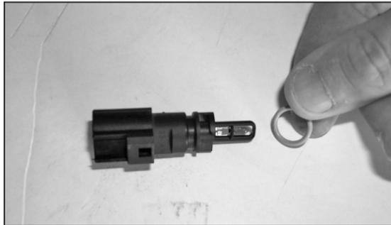
20. Remove the O-ring from the air temp. sensor as shown.
