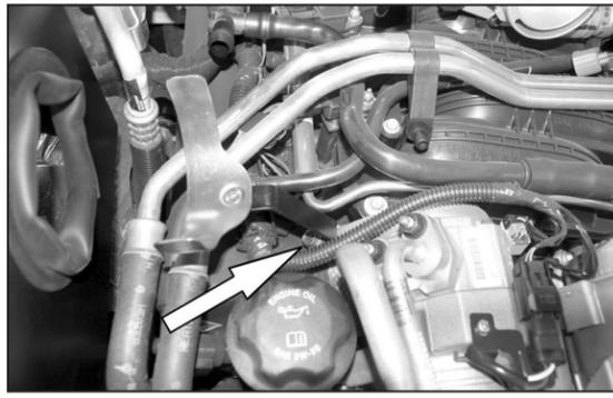
16. Install tube mounting bracket assembly onto A/C compressor using the bolt removed in step #14 as shown.
