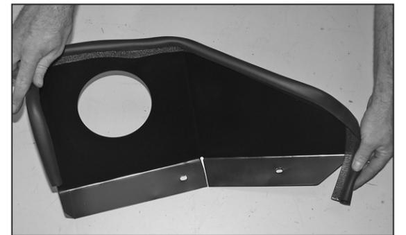
7. Install the provided edge trim onto the heat shield as shown.
