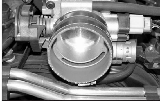
17. Install the provided silicone hose (08690) onto the throttle body and secure with the provided hose clamp as shown.
