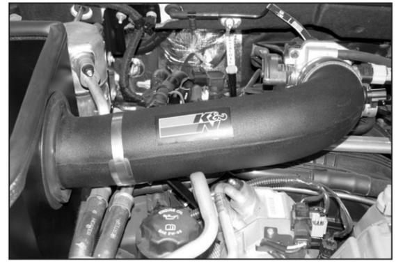
22. Install the K&N® intake tube onto the throttle body hose and position so the tube aligns with the saddle clamp. Secure with the provided hose clamps as shown.
