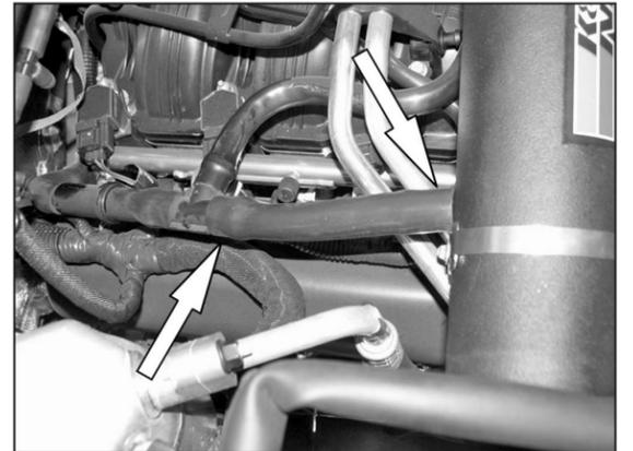
24. Install the provided silicone crank case vent hose onto the factory crank case vent tube and then onto the K&N® intake tube as shown.
