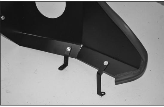
10. Install the "C" bracket (010118) onto the heat shield with the provided hardware as shown.
