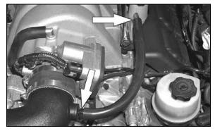
28. Install the provided crankcase vent hose onto the valve cover fitting. Then, connect the open end to the  $\frac{1}{4}$ " NPT fitting installed into the K&N® intake tube.
