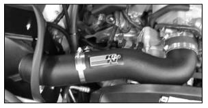
27. Install the K&N® intake tube into the silicone hose on the throttle body and align with the saddle clamp. Then, secure the intake tube with the provided hose clamps.
