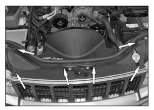
7. Using a small screw driver, release the center holding pins in the six grille retaining clips as shown.
