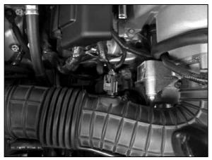
2. Release the red locking tab and disconnect the air temperature sensor electrical connection as shown.
