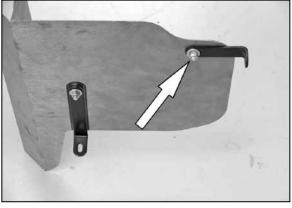
18. Install the small "L" bracket (#07158) onto the heat shield with the provided hardware as shown.
