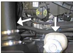
23. Install the provided silicone hose onto the factory crank case vent tube and then connect the open end to the 90° fitting installed into the K&N® intake tube.
