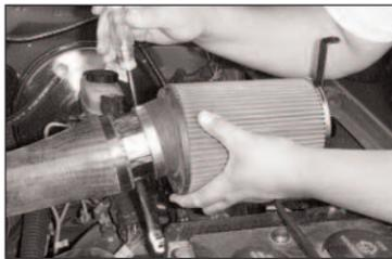
7. Install the filter assembly on to the tube adapter as shown.
