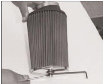
6. Using the hardware provided, install the "L" bracket onto the stud located on the top plate of the air filter.
