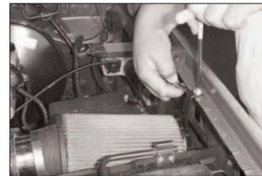
12. Install the filter assembly, lining up the bracket with the previously drilled hole. Secure the bracket with hardware provided as shown in the parts illustration.
