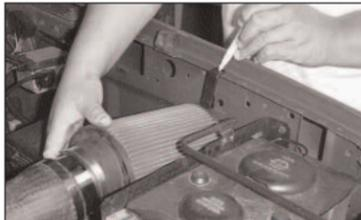
8. Line up the bracket with the fender as shown, then mark the hole.
