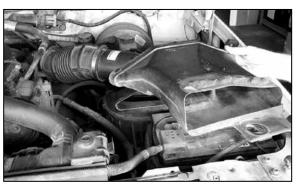
2. Loosen and remove the bolt on the radiator core support, then remove the air inlet duct as shown.
