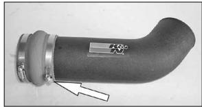
14. Install the silicone hump hose onto the K&N<sup>®</sup> intake tube as shown and secure with the provided hose clamp.
