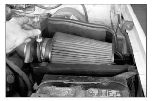
27. Tighten the hose clamp on the K&N® air filter as shown.
