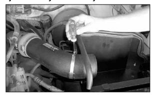
23. Secure the K&N® intake tube to the saddle bracket with the provided hose clamp as shown. NOTE: Do not tighten completely as some adjustment may be necessary.
