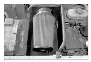
26. Install the K&N® air filter onto the K&N® intake tube, then, line up the stud on the filter with the air filter support bracket and secure with the provided hardware.
