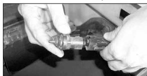
8. Using a small flat blade screwdriver, release the Air Temperature Sensor retaining clips, then disconnect the electrical connection as shown.
