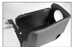
9. Apply the provided trim seal to the K&N® heat shield as shown.
