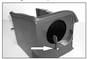
13. Install the saddle bracket assembly onto the  $K\&N^{\odot}$  heat shield using the provided hardware as shown.
