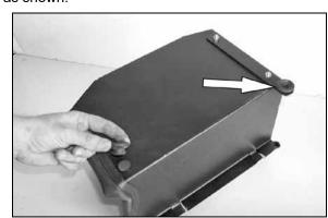
18. Install the stock rubber grommets from the lower air cleaner assembly into the K&N<sup>®</sup> heat shield assembly as shown.
