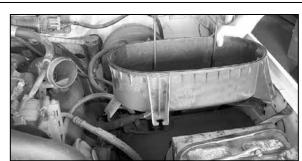
7. Pull firmly upwards to release the lower air cleaner assembly from the retaining grommets, then remove as shown.
