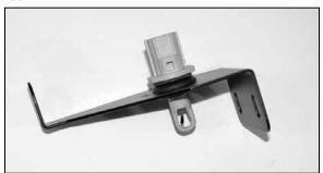
17b. Vehicles that come with twist in air temp sensor, install sensor into air filter support bracket as shown.
