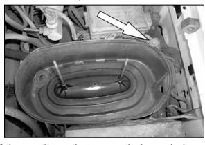
Loosen the nut that secures the lower air cleaner assembly as shown.
