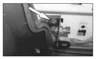
20. Install the air filter support bracket onto the fuse box support bracket using the bolts removed in step 15.
