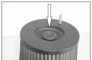
25. Install the grommet that was removed in step 24 into the hole on the top of the K&N® air filter as shown
