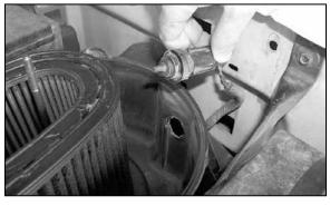
5. To remove the air temperature sensor, turn the sensor ¼ turn, then, pull the sensor out of the lower air cleaner assembly as shown.
