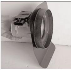
16. Using the provided hardware, assemble the mass air adapter, gaskets, heat shield and mass air sensor as shown.
