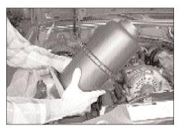
8. Pull firmly up on airbox to release airbox from grommets on the lower support bracket assembly.
