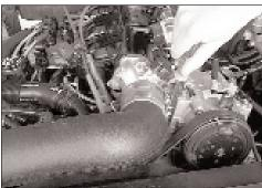
27. Install the K&N® intake tube onto the throttle body and secure as shown.
