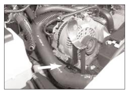
21. Remove the front lower alternator bolt, then secure the saddle bracket assembly using the same bolt as shown.
