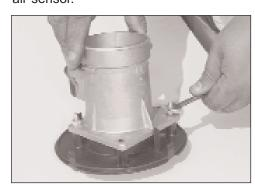
15. Loosen and remove the nuts from the mass air sensor.
