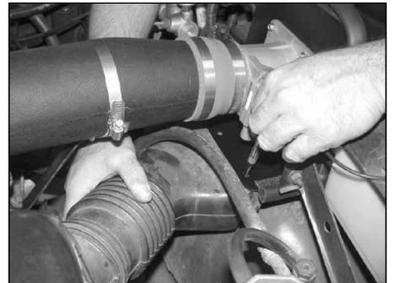
17. Install the mass air assembly onto the intake tube then line up the fresh air duct to the heat shield and mark the two holes with a marker.
