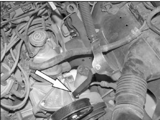
9a. On vehicles that do not come equipped with A/C, mount the saddle bracket assembly from step 8a onto the idler pulley bracket as shown.
