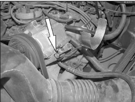
9. On vehicles that come equipped with A/C, remove the front lower A/C mounting bolt. Then secure the saddle bracket assemble from step 8 onto vehicle as shown.
