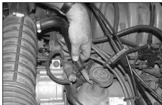
4. Loosen the hose clamp that secures the crank case vent to the calve cover then remove hose.
