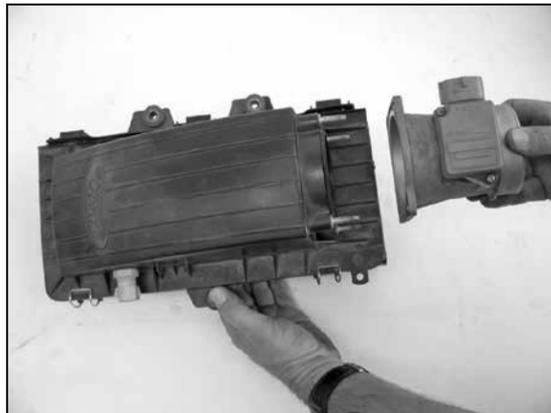
12. Remove the mass air sensor from the factory airbox as shown.
