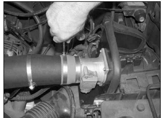
19. Reinstall the mass air assembly and secure with the provided hose clamps.
