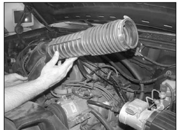
5. Loosen the three hose clamps that secure the intake tube to the air box and throttle body then remove the intake tube.
