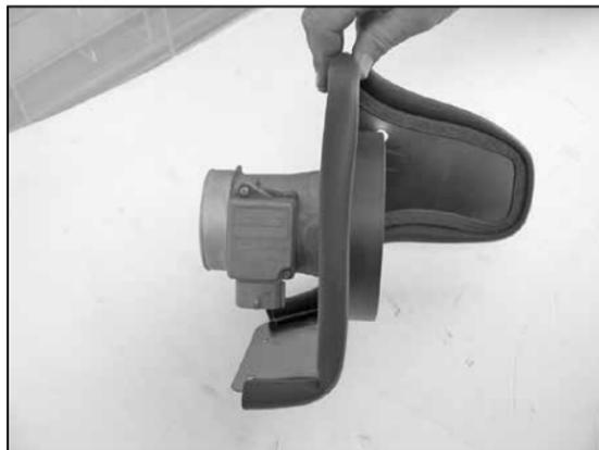
14. Assemble to mass air sensor to the heat shield and filter adaptor using the provided gaskets and hardware as shown.
