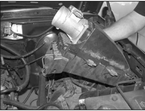
7. Remove the three bolts that secure the air box to the vehicle then remove air box from vehicle.
