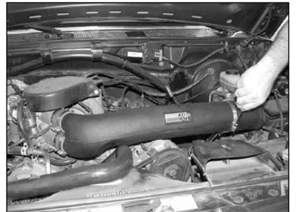
16. Install the new K&N® intake tube onto the throttle body, then secure the intake tube to the saddle bracket as shown.
