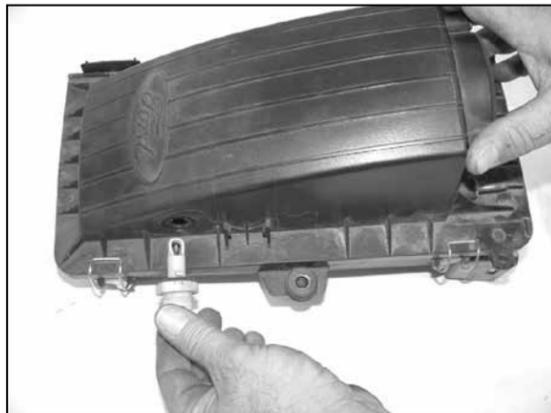
13. Twist the temp sensor counter clock wise to remove from the factory airbox.
