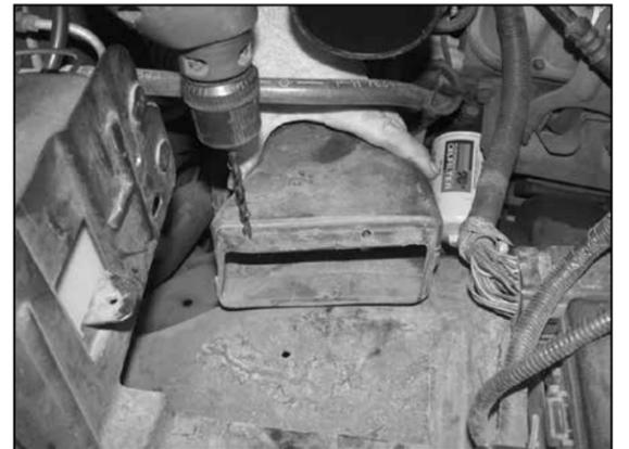
18. Remove the mass air assembly and drill two 1/4" holes were marked in the previous step.
