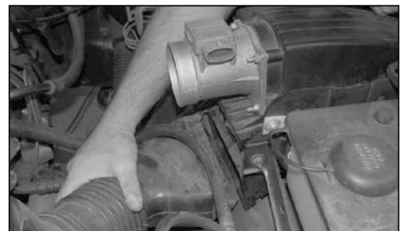
6. Remove the fresh air intake tube from the bottom of air box as shown.
