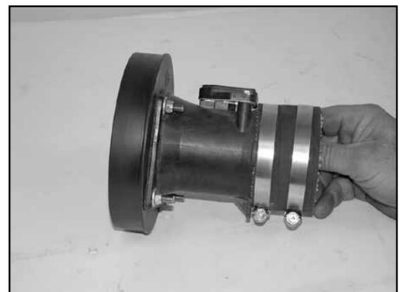
23. Install the silicone hose (08690) onto the mass air sensor with provided hose clamps as shown.
