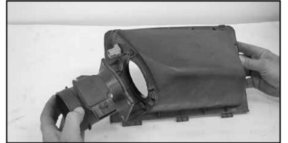
20. Remove the four bolts that retain the mass air sensor to the airbox lid, then remove the mass air sensor from lid.
