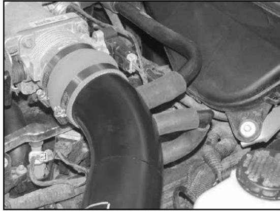
28. Reconnect the crank case vent and idle air hose onto the new intake tube with the provided silicone hoses as shown.
