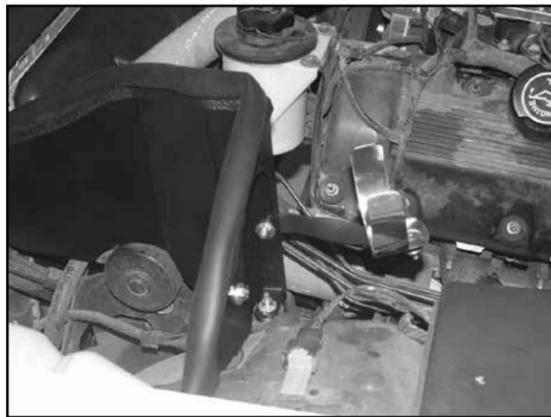
16. Install the saddle bracket assembly onto the heat shield as shown.
