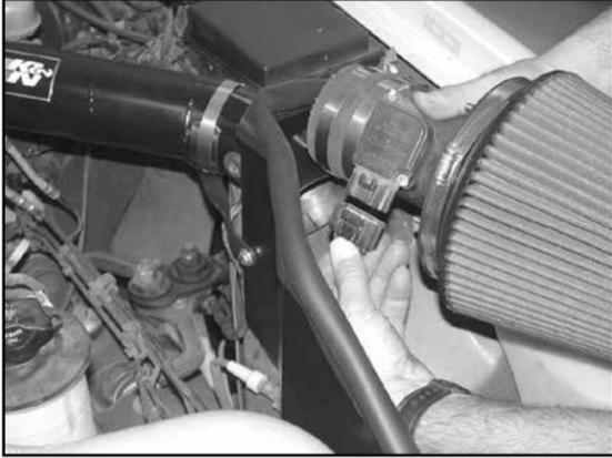
25. Reconnect the mass air sensor electrical connection as shown.
