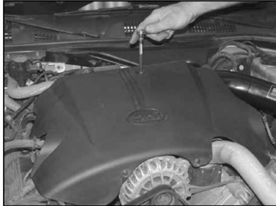
29. Re-install the engine cover that was removed in step 2.
