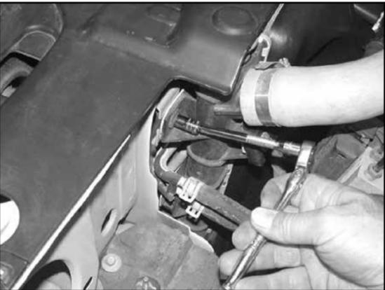
10. Remove the 8mm bolt that retains the radiator fan shroud to radiator.
