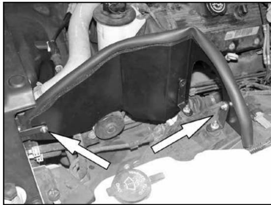
14. Install the heat shield into vehicle and attach to the two outer brackets.
