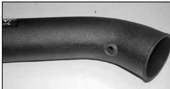
17. On vehicles that come with external temp sensor drill out the drill point with a 3/4 drill, then install the provided grommet as shown.
