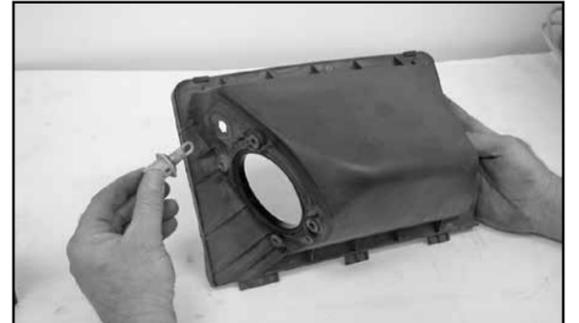
21. On vehicles that come equipped with an external temp sensor, twist counter clockwise to remove from airbox lid.
