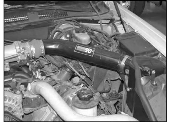
19. Install the K&N® intake onto the throttle body and line it up with saddle bracket assembly.
