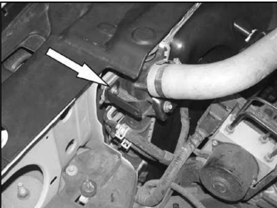
11. Install the provided bracket (07879) onto radiator with the provided hardware.
