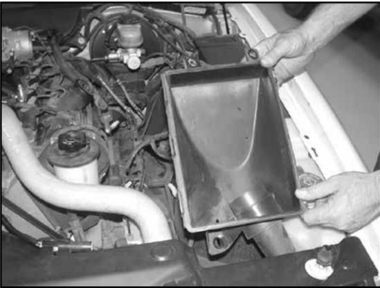
9. Remove airbox bottom from vehicle as shown.
