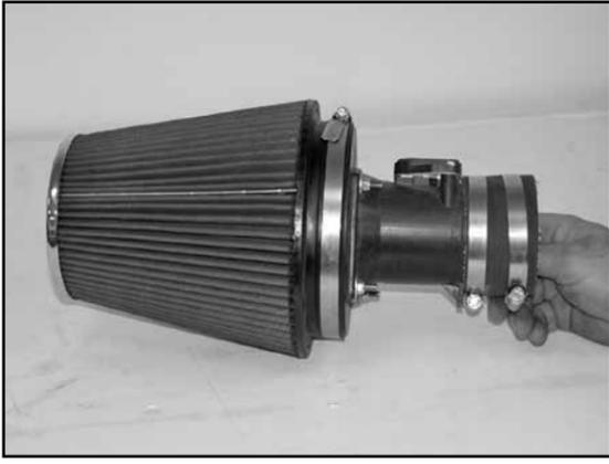
24. Install the filtercharger onto the mass air assembly as shown.
