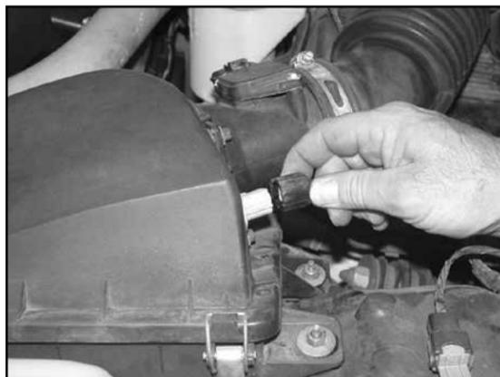
4. Disconnect the temp sensor elctrical connection. **Note: Not all vehicles come with external temp sensors.**
