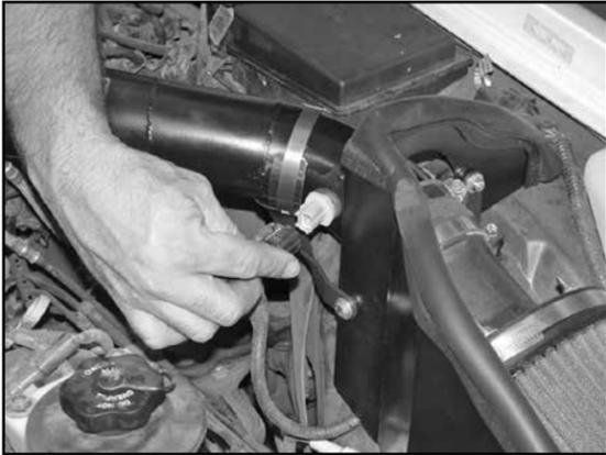
27. On vehicles with external temp sensor, install the temp sensor onto the intake tube then re-connect the electrical connection.
