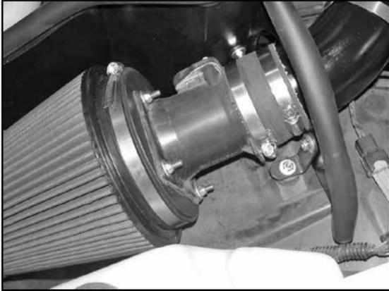
26. Install the mass air assembly onto the intake tube and adjust for best fit before tightening hose clamps.
