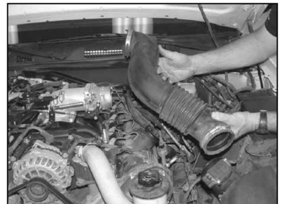
6. Loosen the hose clamp at the throttle body and at the mass air sensor then remove the stock air intake tube as shown.
