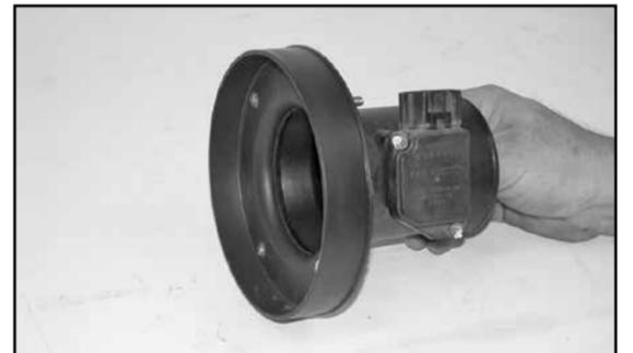
22. Assemble the filter adaptor onto the mass air sensor with the provided hardware as shown.
