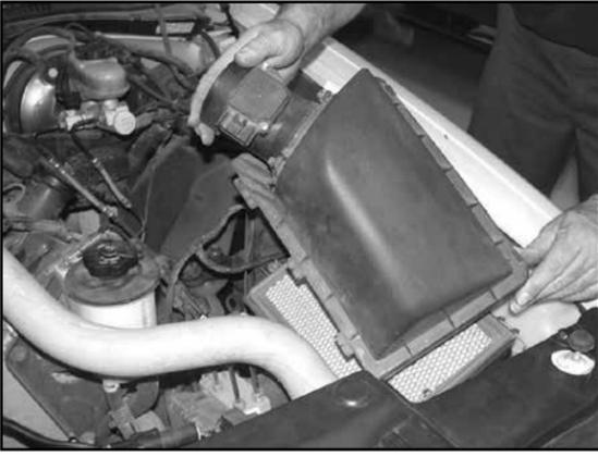
7. Release the 2 clips which retain the airbox lid then remove the lid from the vehicle.
