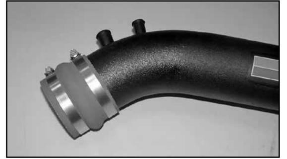
18. Install the provided silicone hump hose (087121) onto the K&N® intake tube with the provided hose clamps.
