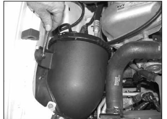
9. Loosen and remove the bolt that retains the air filter assembly onto the vehicle as shown.
