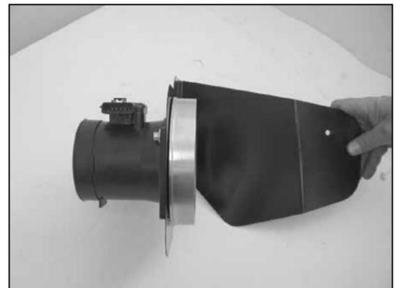
11. Assemble the filter adaptor and heat shield onto the mass air sensor as shown with the provided gaskets and hardware.
