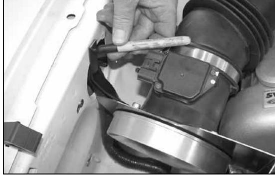
18. Align the bracket to the inner fender then mark the fender with a felt pen.
