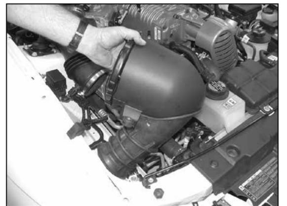
10. Pull the air filter assembly upward and remove from vehicle.
