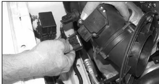
6. Disconnect the mass air electrical connection.
