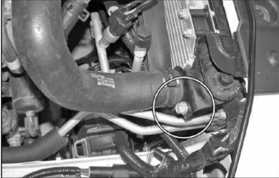
13. Remove the radiator mount bolt with a 13mm wrench.
