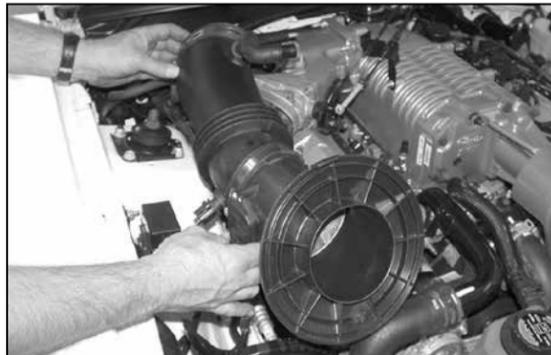
5. Release the intake tube at the throttle body then lift complete intake track up to access the mass air electrical connection.
