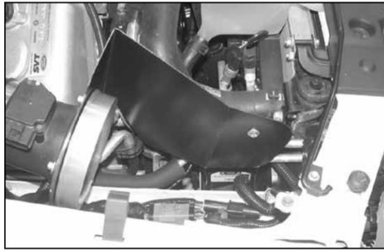
17. Connect the heatshield onto the "L" bracket as shown.
