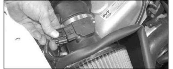
23. Reconnect the mass air electrical connection as shown.
