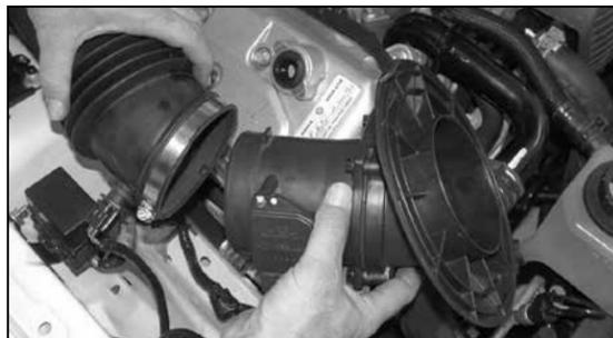
7. Disconnect the mass air from intake tube as shown.
