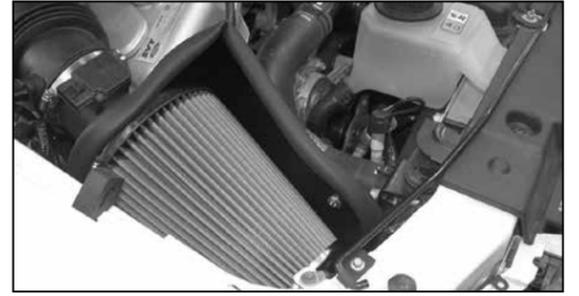
22. Reinstall the mass air assembly onto the intake tube and secure the brackets with the provided sheet metal screw and 6mm bolt onto the "L" bracket.
