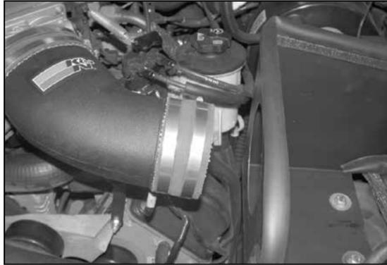
27. Install the silicone hose (08761) onto the intake tube with the provided hose clamps.
