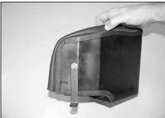
11. Install the "L" bracket onto heat shield as with the provided hardware as shown.
