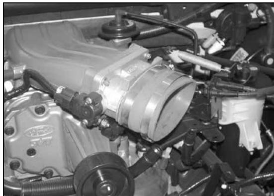
15. Install the silicone hose (08540) onto the throttle body with the provided hose clamp as shown.
