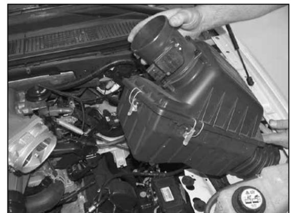
6. Pull up firmly on the factory air box to remove from vehicle. **NOTE: K&N Engineering, Inc., recommends that customers do not discard factory air intake.**
