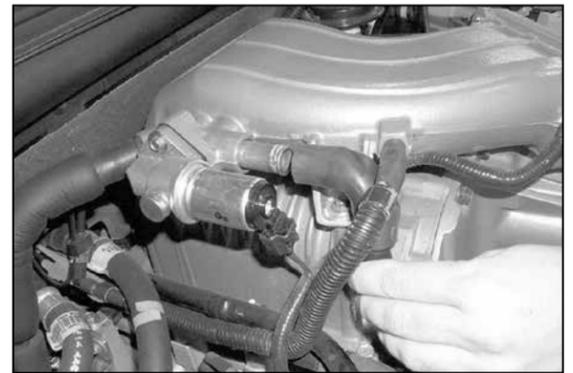
18. Remove the idle air vent tube from vehicle as shown.
