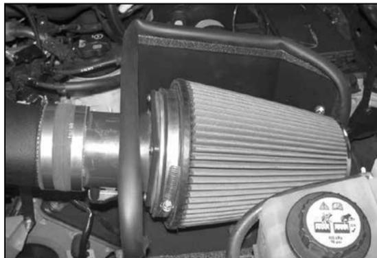
30. Install the Filtercharger onto the mass air adapter and then secure it with the provided hose clamp.
