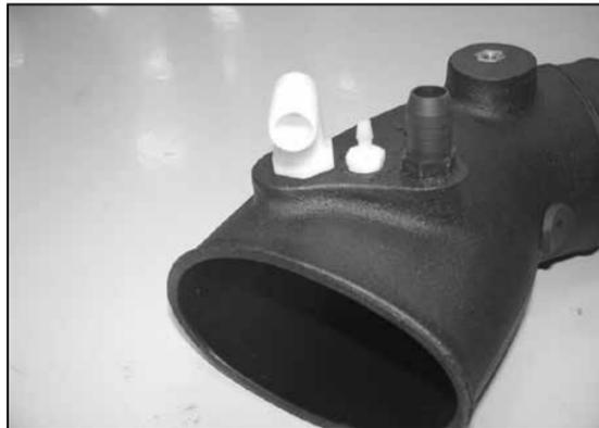
16. Install the provided vent fitting onto the new K&N® intake tube as shown.
