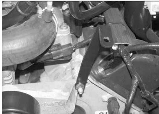
14. Install the provided bracket onto the stud with the nut that was removed in the previous step.
