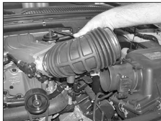
4. Remove the intake tube from vehicle. **NOTE: Disconnect the three vent lines under the intake tube before removing from vehicle.**
