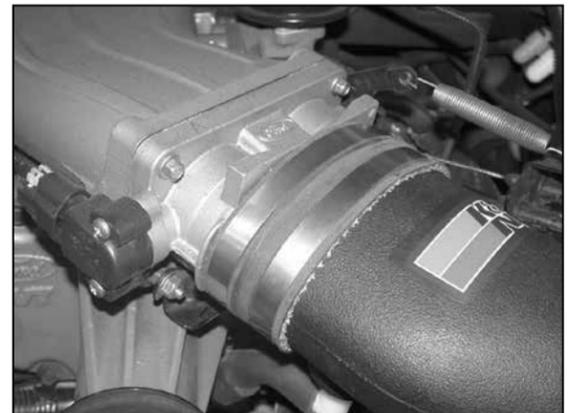
21. Install the new K&N® intake tube into the silicone and then tighten the provided hose clamp.
