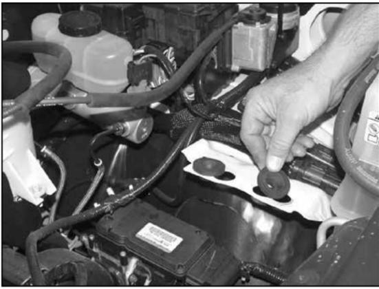
7. Remove the two air box mounting grommets from the air box mounting tray as shown.
