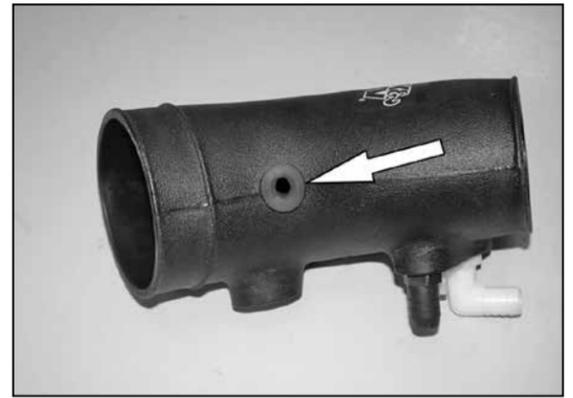
17. Install the provided grommet into the new intake tube as shown.
