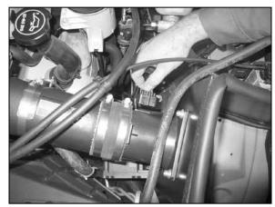
30. Reconnect the mass air sensor electrical connection as shown. Also reconnect the secondary electrical connection
