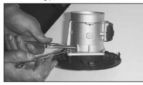
14. Using a pair of small vise grips or pliers, hold the stud while using a 10mm wrench to loosen the nuts, then remove the mass air sensor from the retaining plate.
