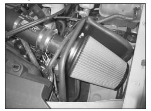
31. Install the K&N<sup>®</sup> air filter onto the mass air sensor assembly as shown.
