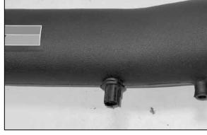
20. Install the air temp sensor into the grommet as shown.
