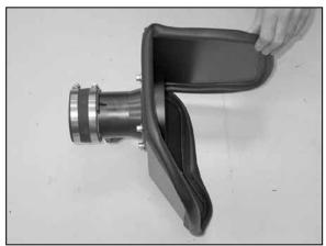
28. Install the silicone hose (08630) onto the mass air sensor.
