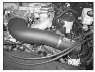
25. Install the new K&N<sup>®</sup> intake tube onto the throttle body and saddle bracket with the provided hose clamps.
