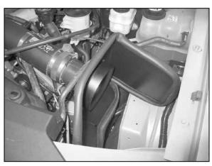
29. Install the mass air assembly onto the K&N<sup>®</sup> intake tube as shown.
