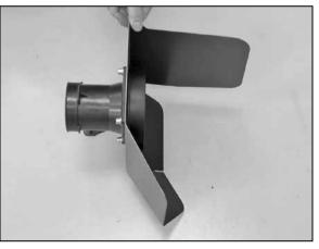
15. Assemble the heat shield and filter adapter onto the mass air sensor with the provided gaskets and hardware.
