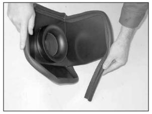
16. Install the edge trim onto the heat shield as shown. Trim if necessary.
