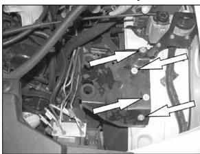
9. Using an 8mm socket, remove the 4 bolts that retain the airbox mounting bracket.
