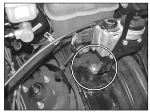
26. Install the provided rubber mounted stud under the cruise control bracket as shown.
