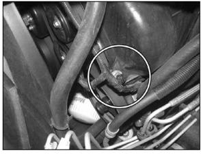
22. Release the wire harness from valve cover stud as shown.
