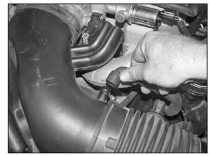
4. Remove the crank case valve hose from the stock intake tube.
