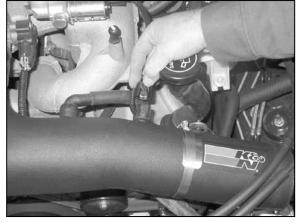
27. Reconnect the crank case valve vent, then reconnect the air temp sensor electrical connection as shown.
