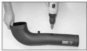
18. On vehicle's equipped with an external air temperature, drill a 5/8"id hole in the K&N<sup>®</sup> intake tube at the drill point as shown.
