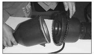
12. Open the air cleaner assembly and isolate the mass air sensor assembly.
