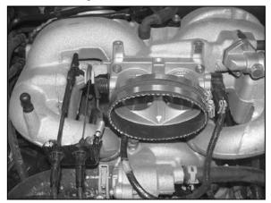
24. Install the silicone hose (08623) onto the throttle body with the provided hose clamps. **NOTE: Be sure to position the worm gears toward the driver side, away from all moving throttle components.**
