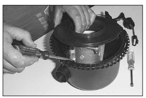
13. Using a flat blade screwdriver, push in and release the four clips that retain the mass air sensor retaining plate.
