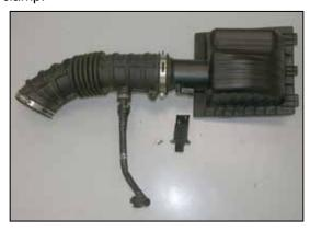
11. Using the "TORX" wrench provided, remove the mass air sensor from the stock airbox assembly as shown.
