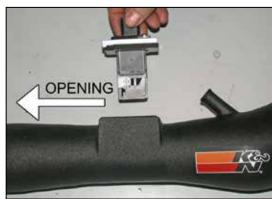
14. Install the mass air sensor assembly into the  $K\&N^{\otimes}$  intake tube as shown.
