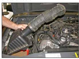
6. Loosen the hose clamp which secures the intake tube to the throttle body, release the two clam shell clamps which secure the upper airbox lid and then remove the airbox lid and intake tube from the vehicle.
