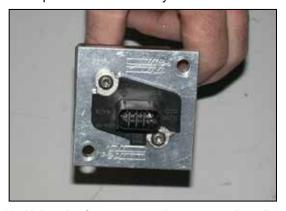
13. Using the factory mounting screws, install mass air sensor into the K&N® adapter assembly as shown.
