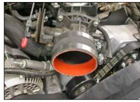
10. Install the silicone hose (08630) onto the throttle body and secure with the provided hose clamp.
