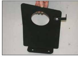
19. Install the heat shield mounting bracket (070742) onto the heat shield with the provided hardware as shown.
