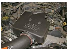
26. Reinstall the engine cover and secure with the factory mounting bolts.
