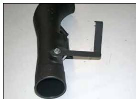
16. Install the provided tube-mounting bracket (010081) onto the K&N<sup>®</sup> intake tube with the provided hardware as shown.
