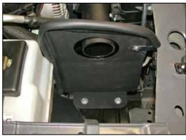
22. Install the heat shield assembly into the vehicle so the bracket lines up with the factory in the core support and the heat shield holes line up with the threaded inserts installed in step #21.
