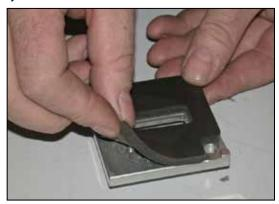
12. Install the provided gasket onto the K&N® mass air adapter as shown. Sticky side down.
