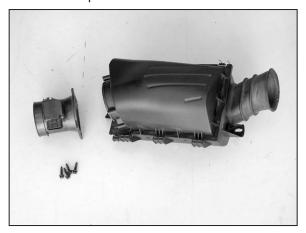
11. Remove the mass air sensor from the air box as shown.
