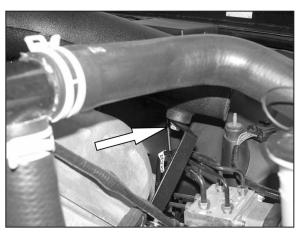
20. Using the provided 8mm bolt, secure the intake tube to the tube-mounting bracket installed in step #17.
