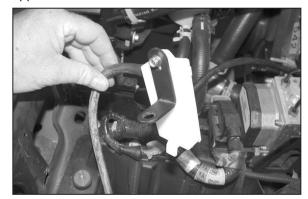
8. Using the provided hardware, secure the muffler to the "L" bracket (070712) as shown.
