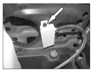
7. Remove the air compressor muffler-retaining pin shown and then remove the muffler from the core support.
