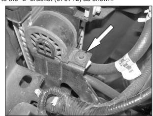
9. Remove the radiator mounting bolt shown.
