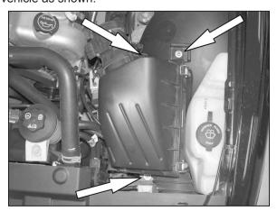
5. Loosen and remove the three air box mounting nuts shown.
