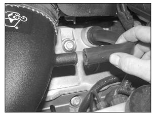
21. Install the supplied silicone vent hose onto the crank case vent fitting in the valve cover and onto the  $K\&N^{\otimes}$  intake tube as shown.
