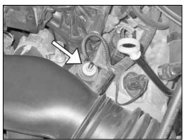
4. Remove the nut which secures the stock intake tube to the mounting stud.
