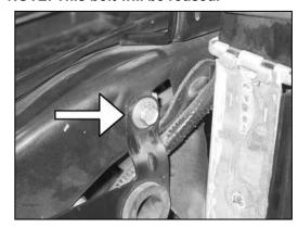
21. Remove the fresh air intake tube mounting bracket bolt shown from the radiator core support. **NOTE: This bolt will be reused.**
