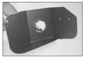
18. Install the short edge trim into the hole in the heat shield as shown.
