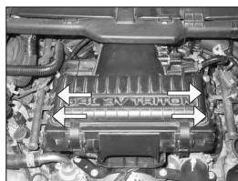
6. Remove the four air filter housing bolts shown.
