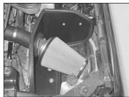
37. Install the filter adapter assembly into the K&N $^{\circ}$  filter and secure with the provided hose clamp.
