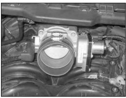
31. Install the silicone hose (08630) onto the throttle body and secure with the provided hose clamp.
