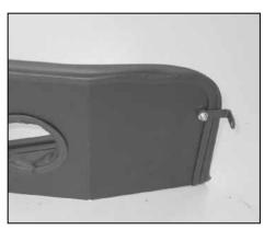
23. Install the small "L" bracket (070812A) onto the heat shield as shown with the provided hardware. NOTE: Be sure to place a flat washer betweeen the heat shield and bracket as a spacer. Do not completely tighten at this time.
