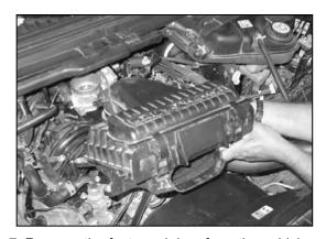
7. Remove the factory air box from the vehicle. NOTE: K&N Engineering, Inc., recommends that customers do not discard factory air intake.
