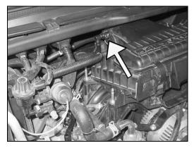
3. Disconnect the crank case vent hose from the factory air box.
