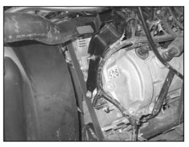
8. Remove the bolt and nut that secure the mounting bracket for the stock fresh air intake tube and then remove the mounting bracket.
