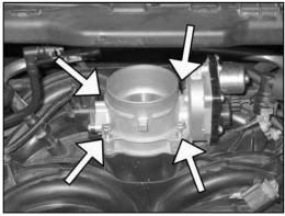
10. Remove the four throttle body mounting bolts. **NOTE: These bolts will be reused.**
