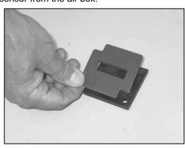
27. Install the provided gasket onto the K&N $^{\circ}$  mass air sensor adapter as shown.
