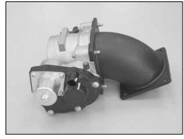
12. Using the factory mounting bolts from step #10, secure the throttle body to the K&N® throttle body adapter with the gasket as shown.
