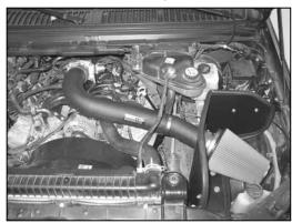
39. Install the filter adapter assembly into the K&N® filter and secure with the provided hose clamp.
