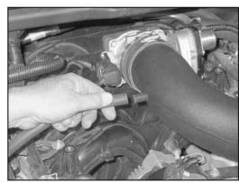
34. Install the supplied crank case vent hose onto the valve cover fitting and then onto the  $K\&N^{\circledcirc}$  intake tube as shown.
