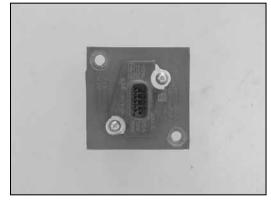
28. Install the mass air sensor into the K&N® adapter and secure with the provided hardware.
