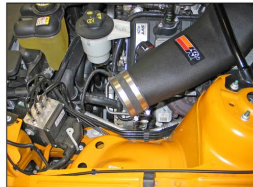
23. Install the silicone hose (08761) onto the intake tube and slide it past the bead on the end of the tube so proper clearance is maintained when the air filter assembly is installed.
