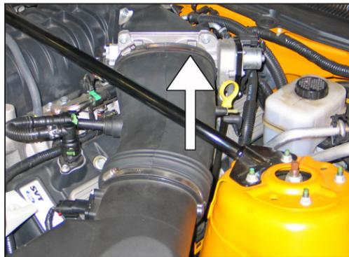
5. Loosen the intake hose clamp at throttle body.
