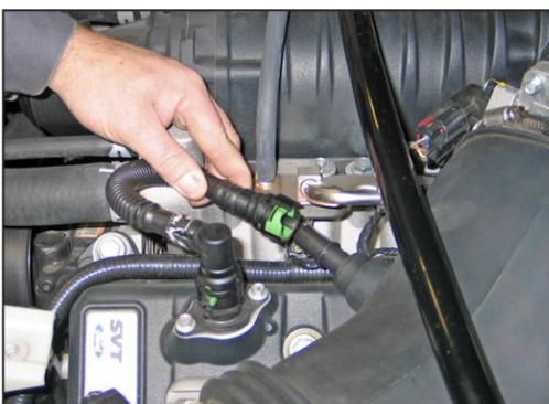
3. Rotate the green locking tab and then disconnect the crankcase vent hose from the intake tube.
