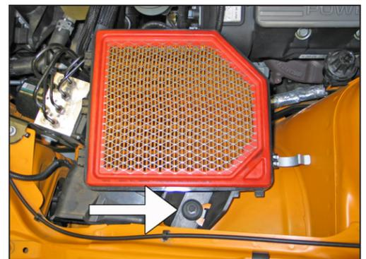
8. Remove the lower airbox retaining bolt shown.
