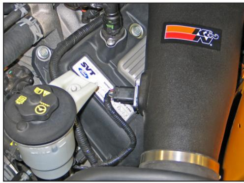
27. Reconnect the mass air sensor electrical connection.
