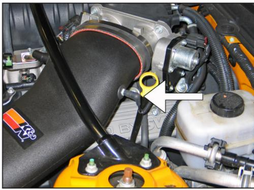
25. Connect the vacuum vent line onto the 1/4" hose mender that was inserted in the K&N® intake tube during step #13.
