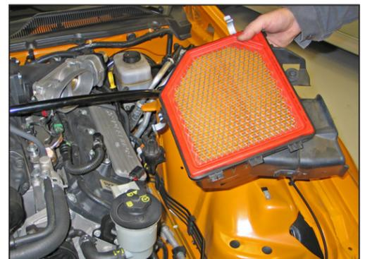
9. Remove the lower airbox housing from the vehicle.
