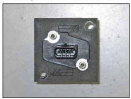
20. Install the mass air sensor into the adapter using the provided bolts.
