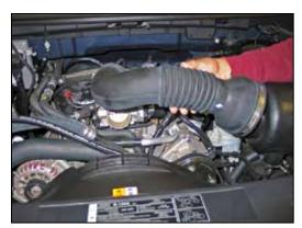
3. Loosen the hose clamps that secure the stock intake tube to the throttle body and air filter housing; remove the intake tube from the vehicle.
