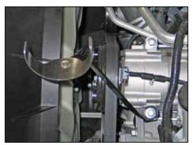
9. Install the tube mounting bracket assembly onto the A/C compressor using the bolt removed in the previous step.
