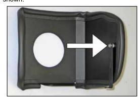
11. Install the heat shield mounting bracket onto the heat shield with the provided spacer and hardware as shown.
