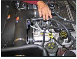
27. Install the supplied crank case vent hose onto the valve cover and secure with the provided hose clamp. Connect the other end onto the intake tube as shown.
