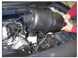
4. Firmly pull up the assembly to unhook it from the mounting grommets and inner fender as shown.
