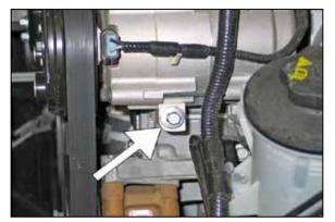
8. Remove the lower front A/C compressor mounting bolt shown.
