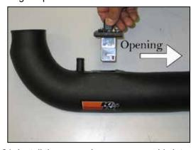
21. Install the mass air sensor assembly into the K&N® intake tube and secure with the provided hardware.
