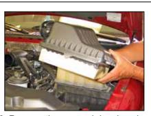
8. Remove the upper air box housing and air filter from the lower air box housing as shown.
