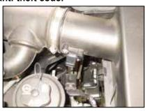
2. Release the red locking tab and disconnect the mass air sensor electrical connection.
