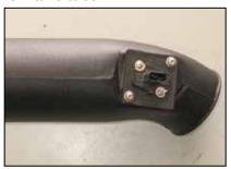
14. Secure the mass air sensor assembly onto the intake tube with the provided hardware as shown.
