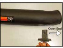
13. Install the mass air sensor assembly into the intake tube.
