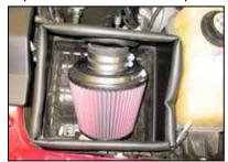
23. Place the air filter assembly into the heat shield as shown.
