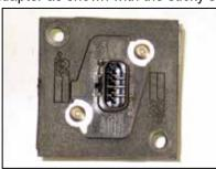
12. Install the mass air sensor onto the mass air sensor adapter with the provided hardware as shown.
