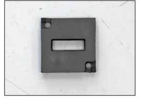
26. Attach the provided gasket onto the mass air sensor adapter as shown.
