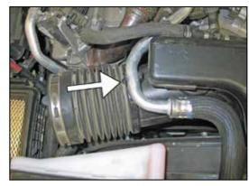
7. Unhook the coolant pipe from the intake tube.
