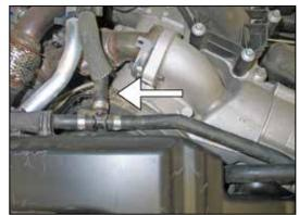
2. Release the red locking tab and then disconnect the mass air sensor electrical connection and unhook the wiring harness from the air box.
