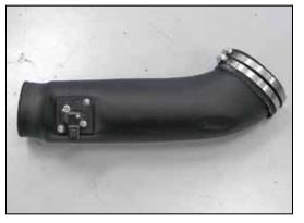
30. Install the provided silicone hose (08540) all the way onto the K&N<sup>®</sup> intake tube so the end of the tube is exposed.
