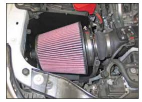
38. Feed the K&N<sup>®</sup> air filter top first into its location, then rotate it back and install onto the filter adapter. Secure the air filter with the provided hose clamp.
