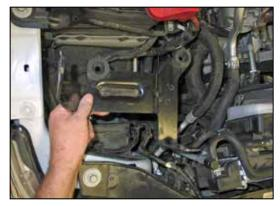
13. Remove the air box mounting bracket from the vehicle.
