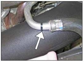
32. Secure the coolant pipe to the insert of the  $K\&N^{\otimes}$  intake tube with the provided mounting tie wrap.
