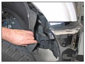
15. Remove the 5 bolts and one push pin securing the front of the inner fender panel and then pull the inner fender panel back to gain access to the bottom of the fresh air intake duct.
