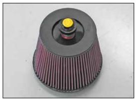
37. Install the filter minder along with the provided grommet into the  $K\&N^{\circ}$  air filter as shown.
