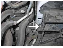
18. Unhook the wiring harness secured to the core support through the fresh air intake duct.
