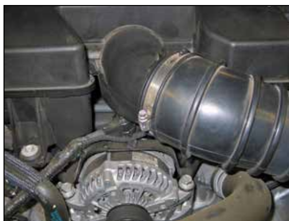
3. Loosen the hose clamp that secures the intake tube to the intake plenum.
