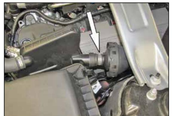
5. Cut the clamp securing the sound tube to the sound drum and then disconnect the sound tube.
