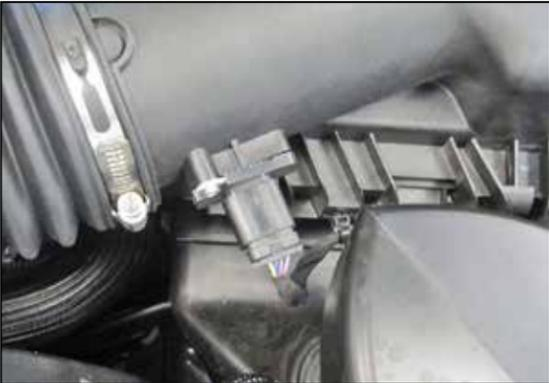
8. Release the red locking tap on the underside of the MAF electrical connector and then disconnect the MAF electrical connection.
