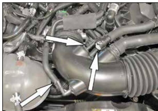
3. Disconnect the Idle by-pass, EVAP vent line and the crank case vent line from the factory intake tube.
