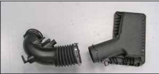
11. Loosen the hose clamp and then remove the factory intake tube from the upper air filter housing.
