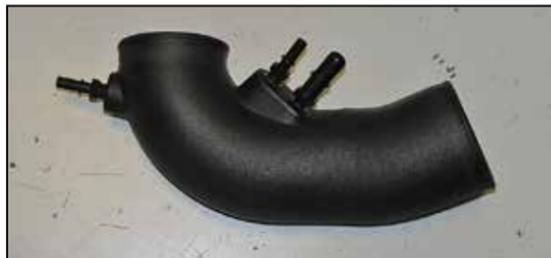
15. Install the three quick disconnect fittings into the K&N® intake tube as shown.
