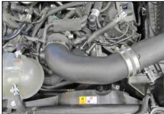
16. Install the K&N® intake tube into the hump hose at the throttle body and then into the coupling hose on the upper air box housing. Secure the hoses with the provided hose clamps.
