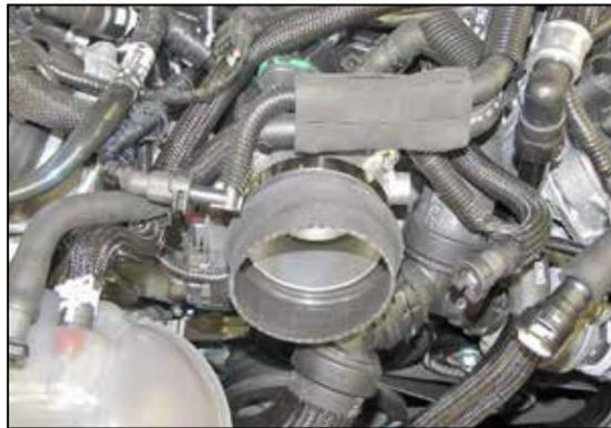
13. Install the provide hump coupler (08699) onto the throttle body and secure with the provided hose clamp.
