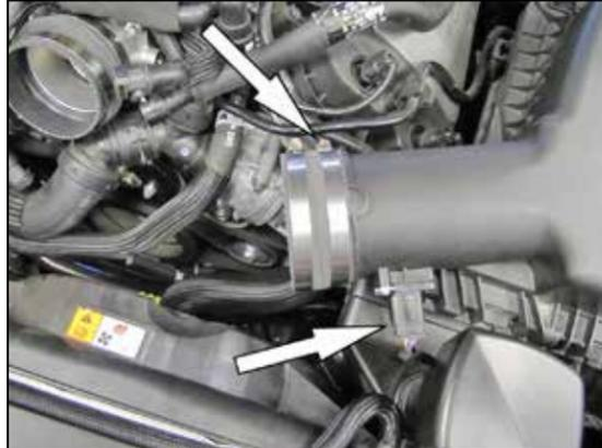
14. Install the provided coupling hose (08760) onto the air filter housing and secure with the provided hose clamp then reconnect the mass air sensor electrical connection.
