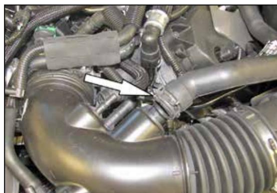
4. Using pliers, squeeze the spring clamp securing the sound tube to the factory intake tube and disconnect the sound tube.
