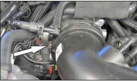
7. Loosen the hose clamp securing the intake tube to the throttle body.
