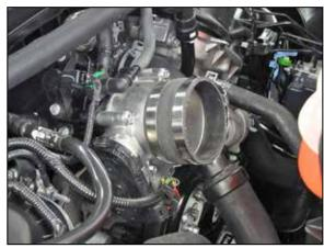
13. Install the provided coupling hose (08699) onto the throttle body and secure with the provided hose clamp.
