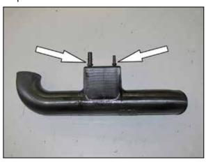
14. Install the two provided quick disconnect fittings into the K&N® intake tube as shown.
