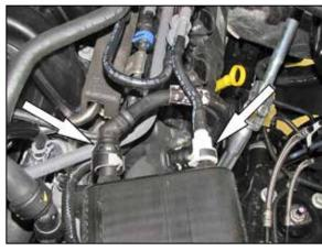
16. Connect the factory EVAP and Crank case vent lines to the fittings on the K&N® intake tube.
