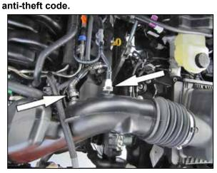
2. Disconnect the EVAP vent connection and crank case vent connection.
