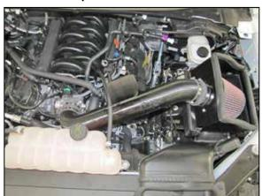
15. Install the K&N® intake into the coupling hose at the filter adapter and then into the hose at the throttle body, adjust the tube for best fit and then secure with the provided hose clamps.
