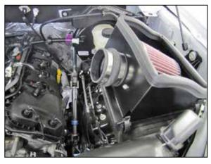
12. Install the provided coupling hump hose (08639) onto the filter adapter and secure with the provided hose clamp.
