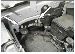
5. Remove the two bolts shown that secure the air filter housing bracket to the inner fender and then remove the bracket from the vehicle.
