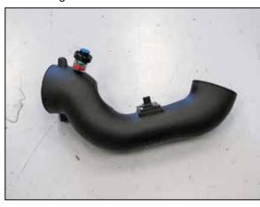
18. Install the filter minder using the provided grommet into the K&N® intake tube.
