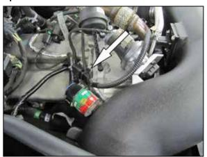
21. Connect the provided mass air sensor extension harness to the factory wiring harness and then into mass air sensor. Using the provided tie wrap, secure the extension harness to the factory harness so that it does not interfere with and potentially moving parts as shown.
