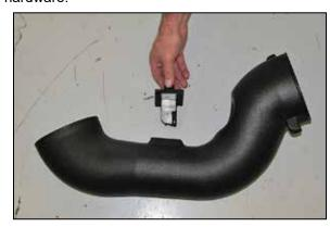
16. Install the mass air sensor assembly into the K&N® intake tube as shown and secure with the provided hardware.
