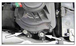
4. Remove the two filter housing mounting bolts shown and then remove the complete air filter housing from the vehicle.
