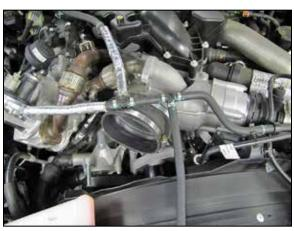
12. Install the provided coupler hose (08695) onto the turbo inlet and secure with the provided hose clamp.
