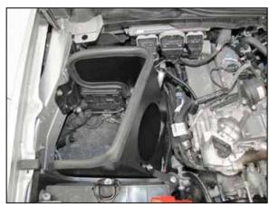
11. Install the heat shield into the vehicle so that the mounting studs insert into the factory air filter housing mounting grommets.
