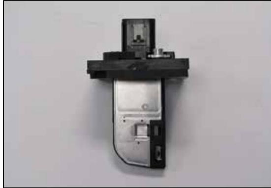
15. Remove the mass air sensor from the factory air filter housing and install it into the mass air adapter using the provided hardware. Install the provided gasket onto the K&N® mass air adapter.
