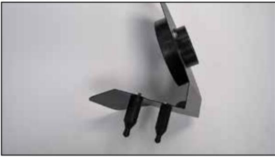
8. Install the two provided heat shield mounting studs onto the heat shield and secure with the provided hardware.
