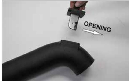
16. Install the mass air sensor assembly into the K&N® intake tube as shown and secure with the provided hardware.
