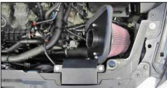
12. Install the heat shield assembly so the mounting studs insert into the air filter housing mounting grommets. Secure the fresh air duct with the hardware provided to the core support and the hardware installed into the heat shield.
