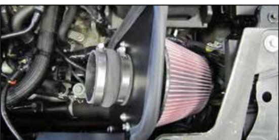
13. Install the provided hump coupler (08699) onto the filter adapter and secure with the provided hardware.
