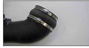
14. Install the coupling hose (08695) and hose clamps onto the intake tube and slide it on as far as possible, do not secure.
