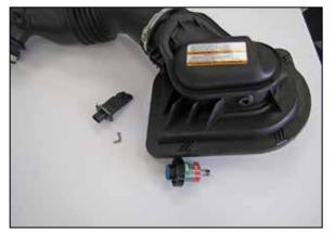
10. Remove the mass air sensor and filter minder from the factory intake tube.
