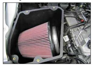
8. Using caution, set the K&N<sup>®</sup> air filter into the K&N<sup>®</sup> air filter housing.
