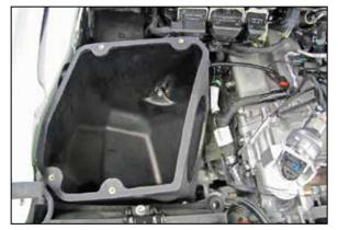
7. Install the K&N<sup>®</sup> air filter housing into the vehicle so that the mounting stud sets into the factory mounting grommet, then using the factory mounting bracket bolt and provided spacer, secure the housing to the inner fender.
