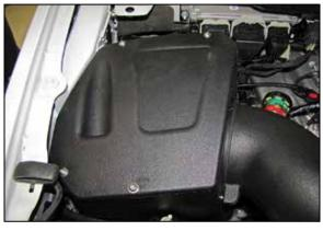
17. Install the air filter housing lid and secure with the provided hardware.
