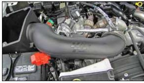
15. Install the K&N<sup>®</sup> intake tube into the K&N<sup>®</sup> air filter housing and align with the turbo inlet. Slide the coupling hose onto the inlet, adjust the tube for best fit and then secure with the provided hardware and hose clamps.
