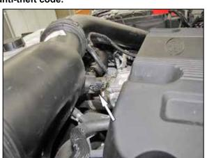
2. Disconnect the inlet air temperature sensor.
