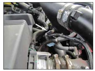
10. Reconnect the inlet air temperature sensor electrical connection.
