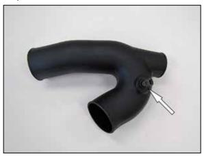
8. Remove the inlet air temperature sensor from the factory intake tube. Remove the O-Ring from the inlet air temperature sensor and then install the sensor into the K&N® intake tube using the provided grommet.
