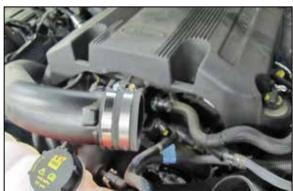
7. Install the provided coupler hoses onto the turbo inlet tubes and secure with the provided hose clamps.
