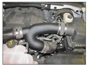
9. Install the K&N® intake tube assembly into the couplers and adjust for best fit, then secure the tube with the provided hose clamps.
