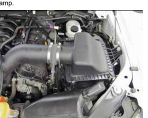
8. Install the K&N<sup>®</sup> intake tube into the coupler at the air filter housing and then into the coupler at the throttle body, adjust the tube for best fit and then secure with the provided hose clamps.
