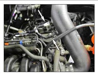
9. Connect the EVAP and crank case vent lines to the quick connect fittings installed into the K&N<sup>®</sup> intake tube.
