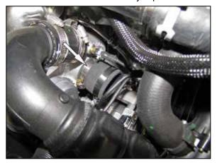
6. Install the provided coupling hose (08638) onto the turbo inlet and secure with the provided hose clamp.
