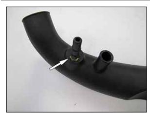
7. Install the provided quick disconnect fitting into the K&N® intake tube as shown.
