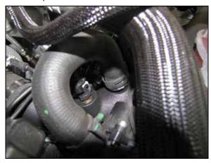
9. Connect the BOV hose and crank case vent hoses to the K&N® intake tube.
