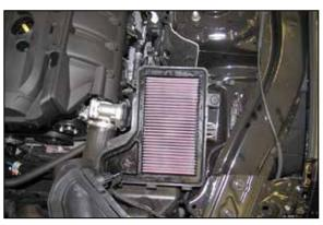
5. Release the clips that secure the upper air filter housing, remove the housing and factory air filter. Install the provided K&N® air filter and then reinstall the lid and secure with the factory clips.
