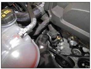
4. Disconnect the BOV hose and crank case vent line from the factory intake tube and then remove the tube from the vehicle.
