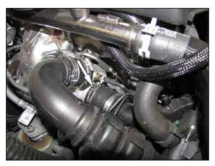
3. Loosen the hose clamp that secures the factory intake tube to the turbo inlet.
